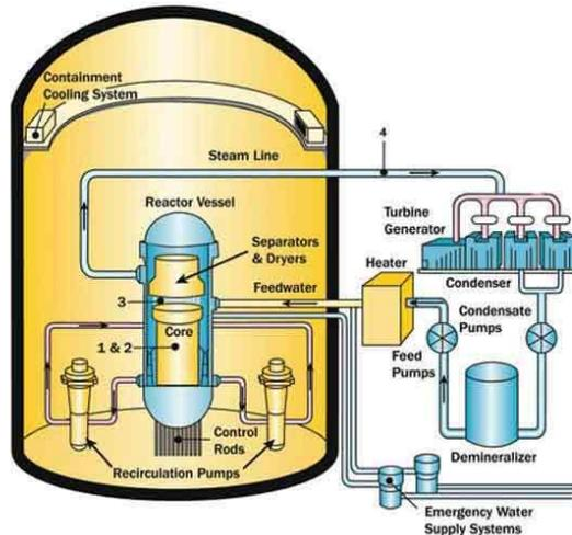
**Figure 3: Typical Boiling Water Reactor Configuration (Source: US Nuclear Regulatory Commission).**
