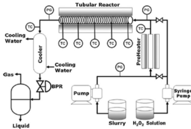
Figure 30. Schematic representation of a Super-Critical Thermal Oxidation system [RHU *et al.*, 2003].
