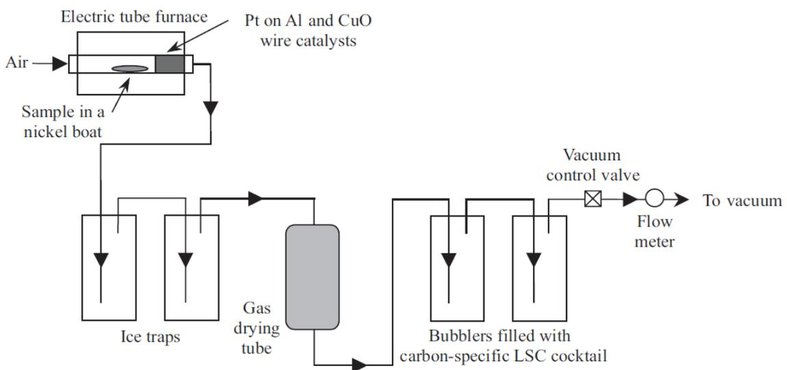
**Figure 26. Schematic of a typical combustion method [MARTIN *et al.*, 1993]**
