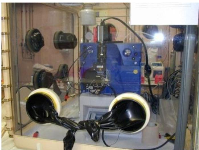
**Figure 33. Electrospray-Mass spectrometry set-up available in CEA.**
