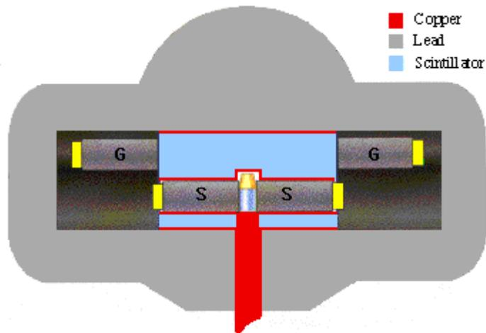
**Figure 17. Internal shielding (active and passive) in a commercial LSC instrument.**
