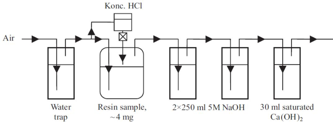
**Figure 24. Schematic representation of an acid stripping system [AITTOLA AND OLSSON, 1980].**
