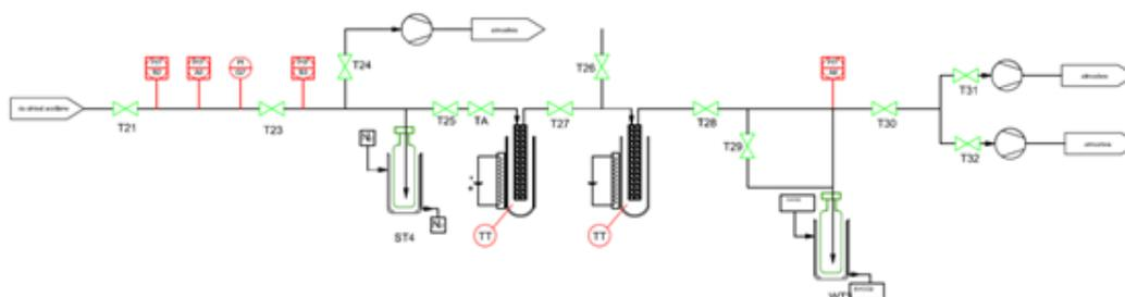
**Figure 16. Schematic representation of the synthesis of benzene at ENEA <sup>14</sup>C laboratory.**
