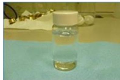
**Figure 20. Vial containing carbamate solution ready to be counted by LSC.**
