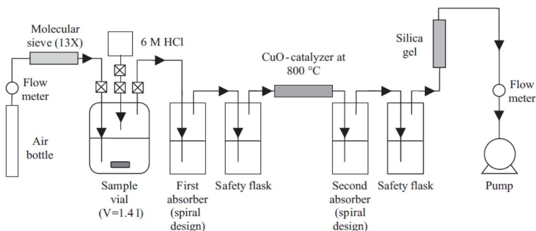
**Figure 28. Schematic representation of a two steps absorption process [SALONEN AND SNELLMAN, 1981].**
