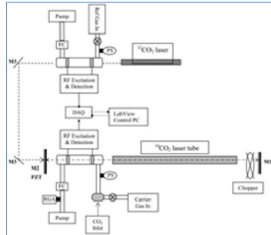
**Figure 23. Scheme of the ICOGS technique**
