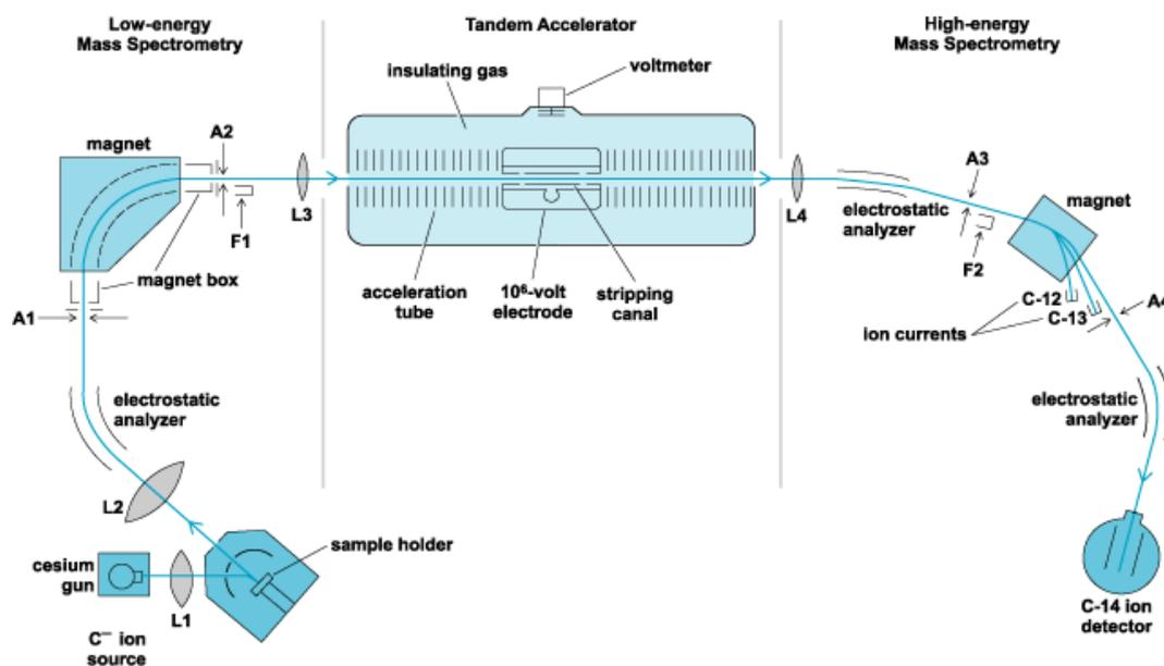
**Figure 14. Schematic drawing of an accelerator mass spectrometer (AMS) used for radiocarbon dating. The equipment is divided into three sections. Electric lenses L1–L4 are used to focus the ion beams; apertures A1–A4 and charge collection cups F1 and F2 are used for setting up the equipment [MCGRAW-HILL, 2007].**
