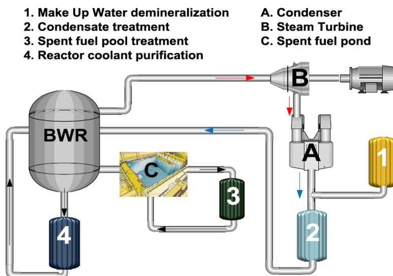
**Figure 4: Water Treatment Circuits with IERs in a BWR [WOLFF, 2012]**
