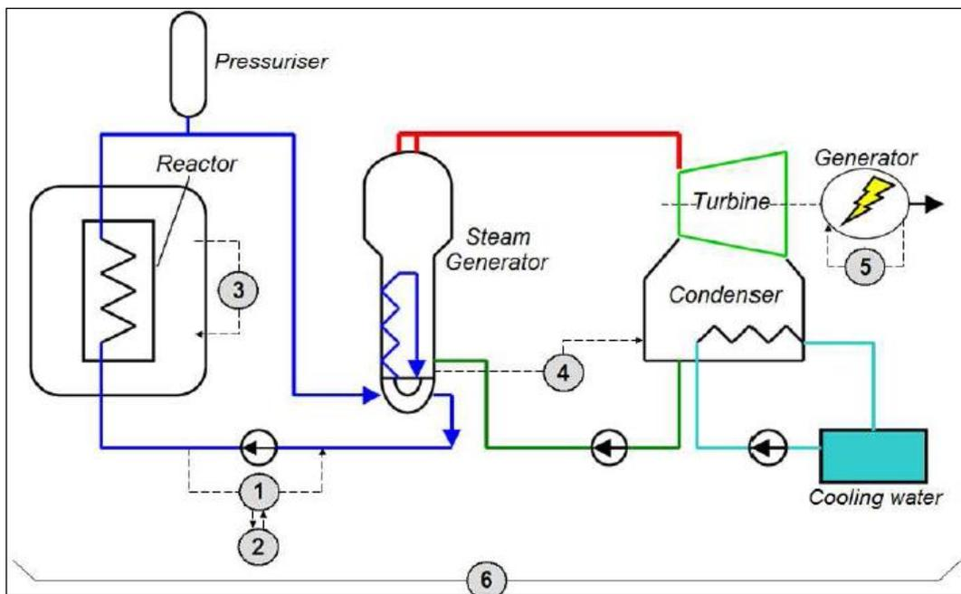
**Figure 1. General location of the key purification systems on an EDF PWR.**
