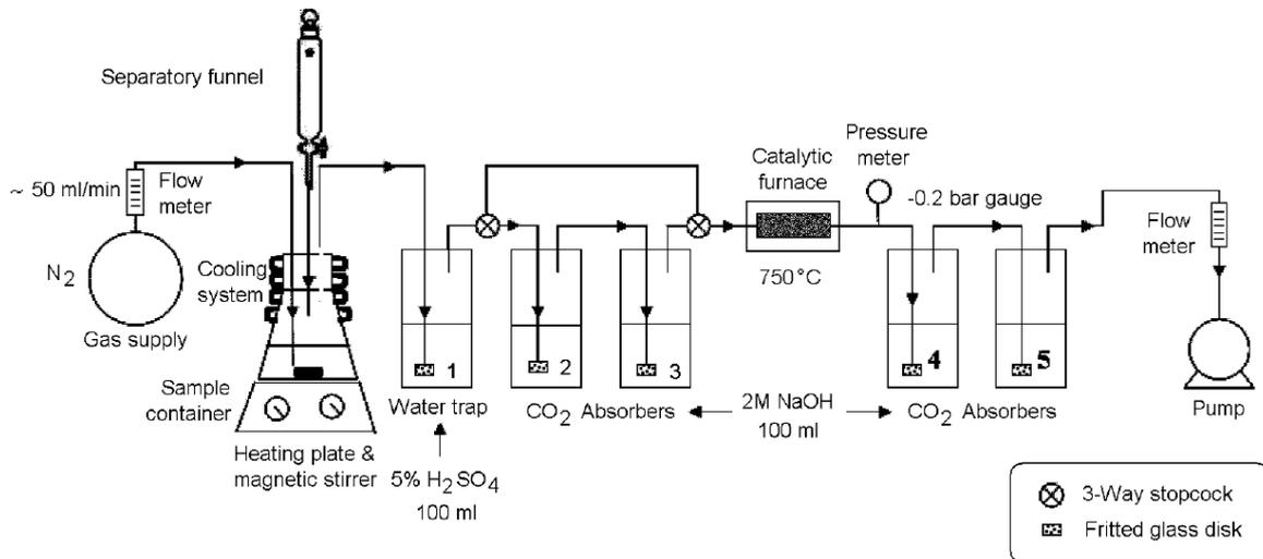
**Figure 29. Schematic representation of double step separation equipment**
