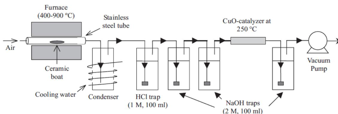
**Figure 27. Combustion scheme used by SPERANZINI AND BUCKLEY [1981].**
