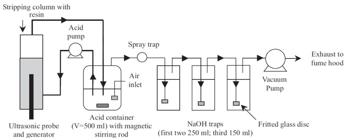
**Figure 25. Schematic representation of an acid stripping system with acid circulation pumping [NOTT, 1982].**
