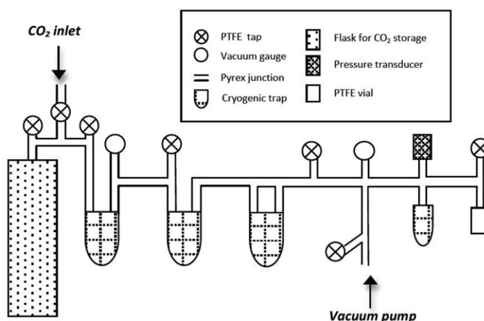
**Figure 21. Equipment for the CO<sub>2</sub> direct absorption method at ENEA <sup>14</sup>C laboratory**
