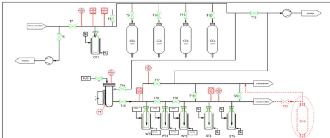
**Figure 15. Schematic representation of the synthesis of acetylene at ENEA  $^{14}\text{C}$  laboratory.**
