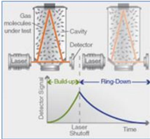
**Figure 22. Basic principle of the Cavity ring-down spectroscopy**
