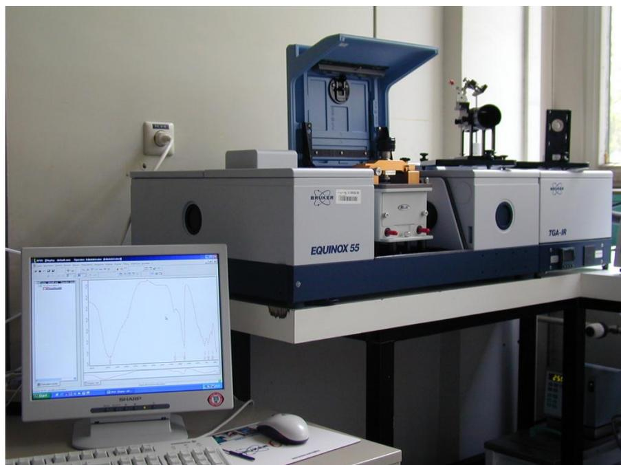
**Figure 34: FTIR Spectrometer coupled with a TGA, available in FZJ.**
