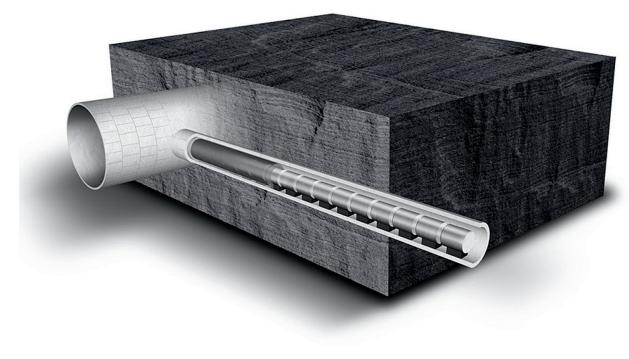
C-14 is present in Zircaloy hulls and end-pieces which are separated from spent fuel and compacted in standard waste containers: CSD-C Colis Standard de Déchets – Compactés. Upon their final disposal the CSD-C containers will be conditioned in concrete Supercontainers and emplaced in disposal galleries of the OPERA disposal concept in Boom Clay host rock.
