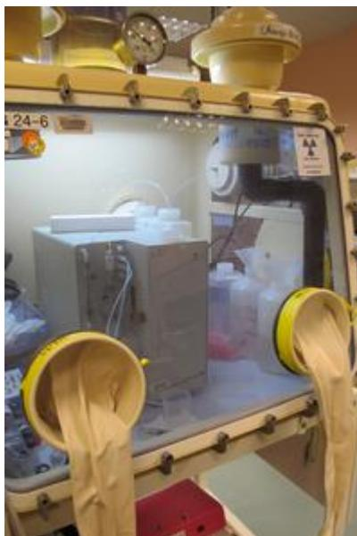
**Figure 2: Total organic carbon analyser implemented in active glove box.**
