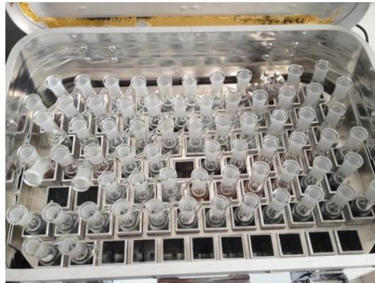
**Figure 12: Metallic box used for the irradiation campaign, loaded with sample vials**
