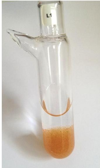
**Figure 11: Sample vial filled with anion exchange resins and water, after closure in controlled atmosphere and pressure, ready for the irradiation campaign**
