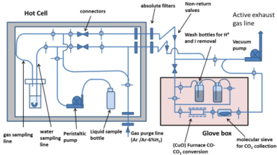
**Figure 22** Schematic diagram of the hot cell testing and sampling glove box for subsequent analysis by liquid scintillation counting
