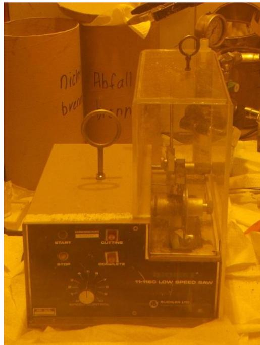
Figure 4 Low speed saw for cutting of Zry-4 specimens under Ar atmosphere in the shielded box-line of KIT-INE.
