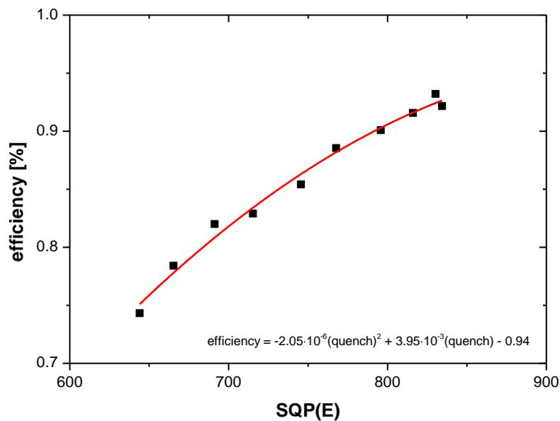
Figure 10 Quench correction curve obtained for 3 mL 2 M NaOH + 18 mL Hionic Fluor
