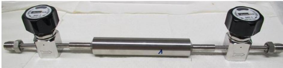
**Figure 8** Two valves gas collecting cylinder for gaseous aliquots of experiments with Zry-4 specimens
