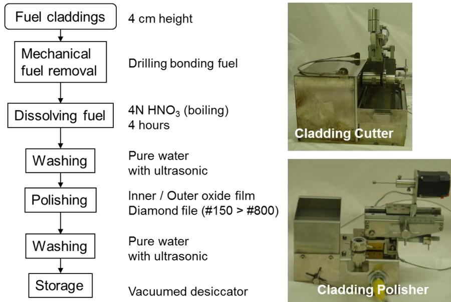
**Figure 13** Pretreatment for Zry-2 specimens
