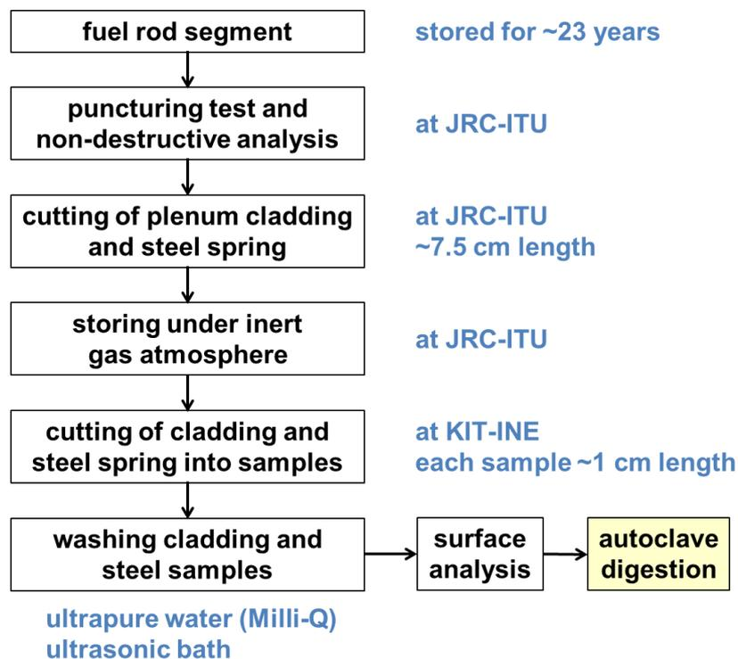
Figure 3 Sample preparation scheme of Zry-4 specimens
