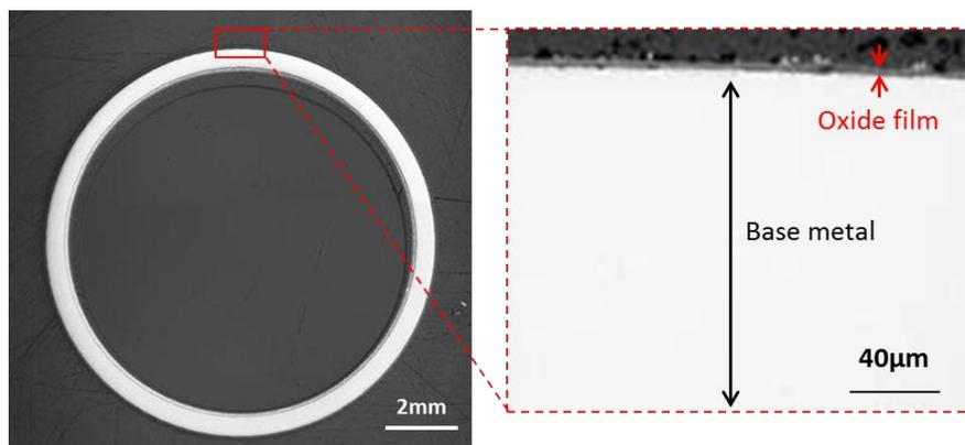
**Figure 14** Picture of Zry-2 specimen before polishing
