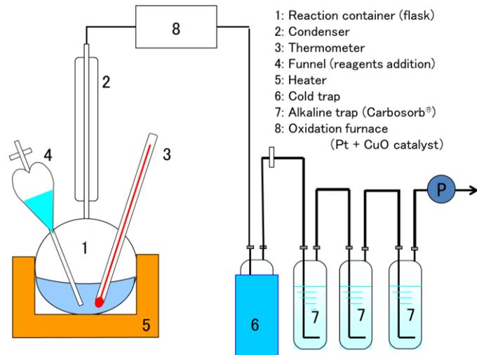
**Figure 20** Apparatus of C-14 analysis in liquid samples
