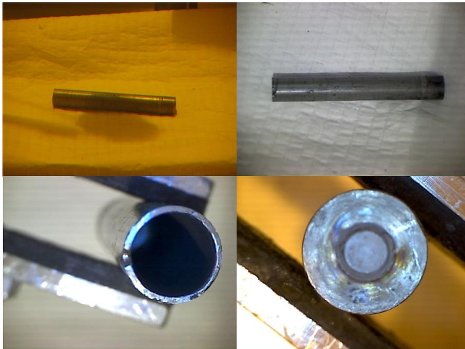
Figure 1 Irradiated Zry-4 plenum specimen used for the dissolution experiments
