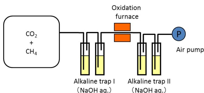
**Figure 19 Outline of the equipment for separating CO<sub>2</sub> and CH<sub>4</sub>**
