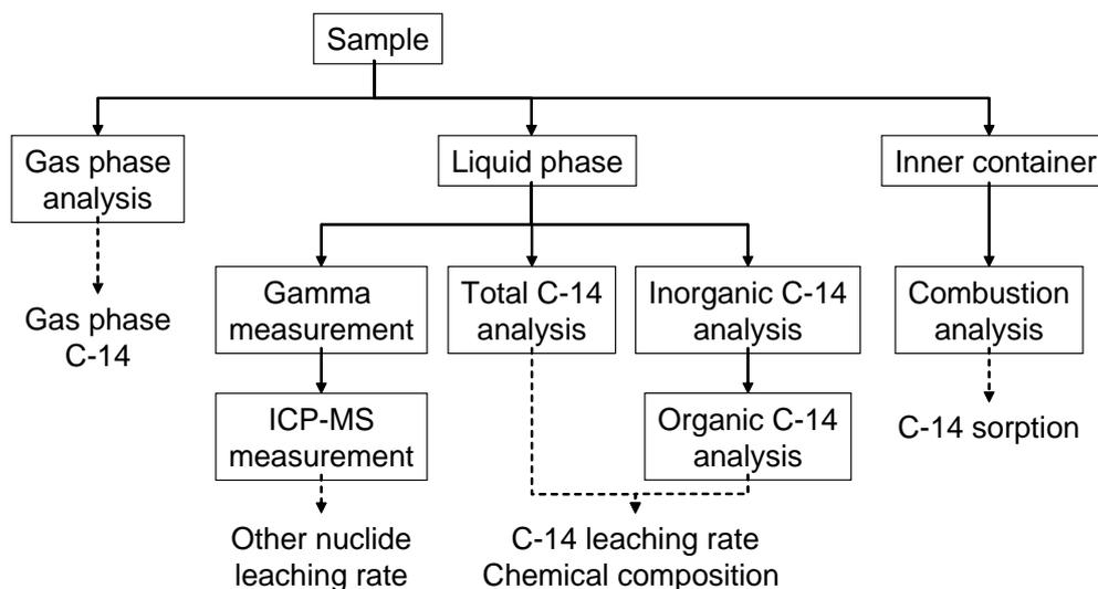
**Figure 17** Flowchart of analysis procedure for leaching test
