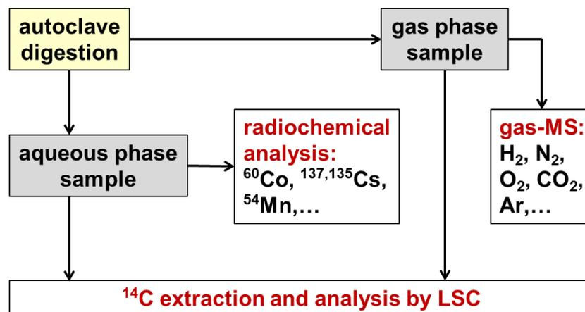
**Figure 5** Scheme of the experimental procedure for quantification of C-14 species of Zry-4 specimens
