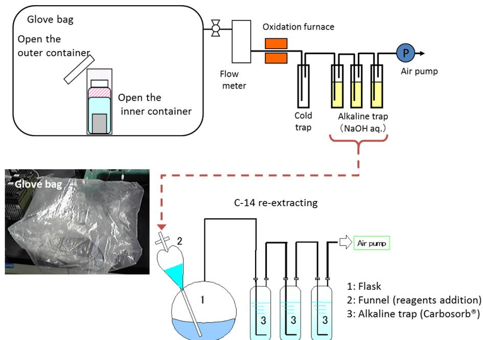
**Figure 18 Outline of apparatus for gaseous total C-14 analysis**
