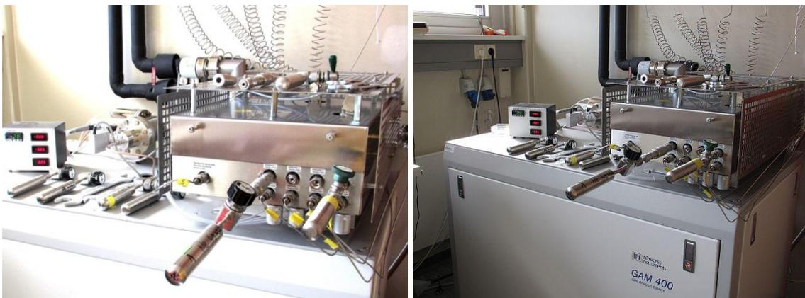
Figure 12 Image of GAM400 quadrupole gas-MS and the batch inlet system
