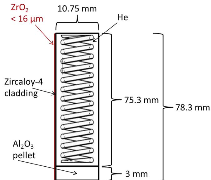
Figure 2 Scheme of the Zry-4 cladding with the stainless steel plenum spring inside
