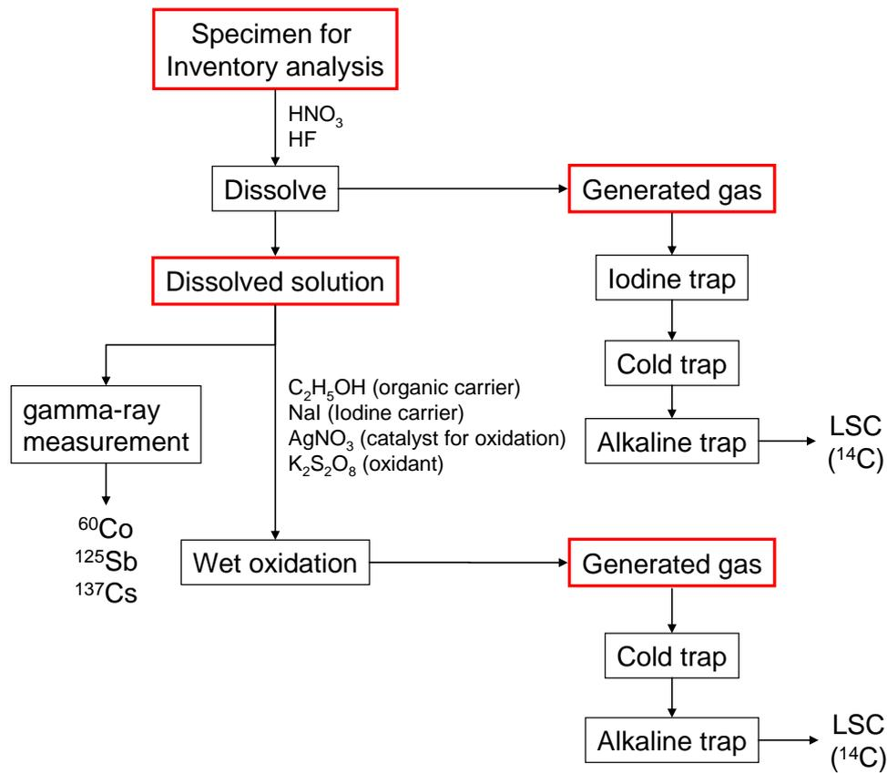
Figure 15 C-14 inventory analysis flow applied for Zry-2 specimens
