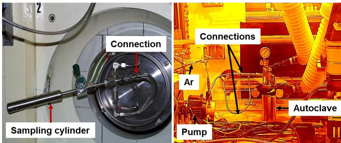
Figure 11 Gas sampling at the KIT-INE shielded box line
