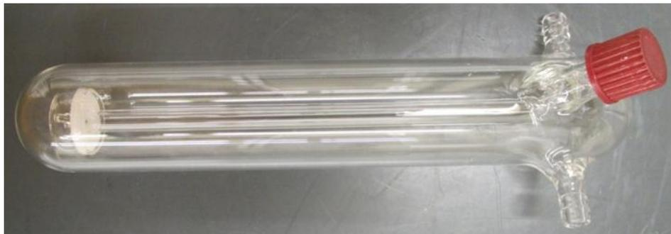
**Figure 9** Customized washing bottle equipped with a fritted glass tip of porosity 1
