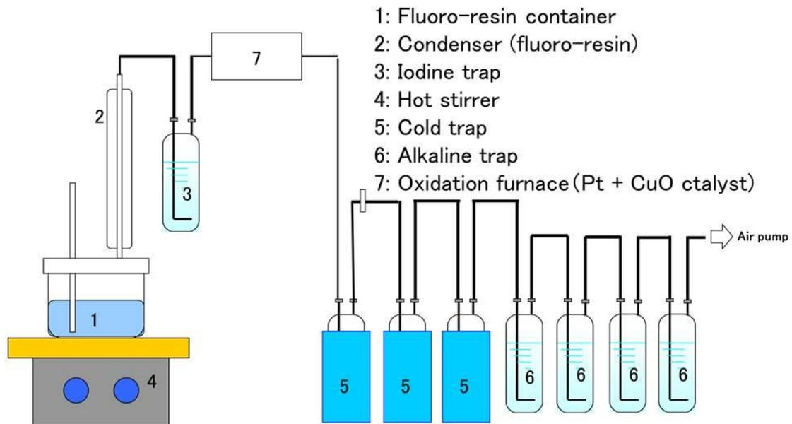
Figure 16 Outline of inventory measuring apparatus for quantification of C-14 of Zry-2 specimens
