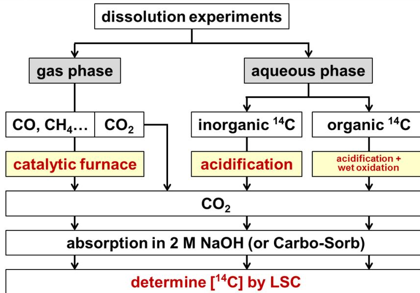
Figure 6 Scheme of C-14 extraction procedure for gaseous and dissolved aliquots of experiments with Zry-4 specimens
