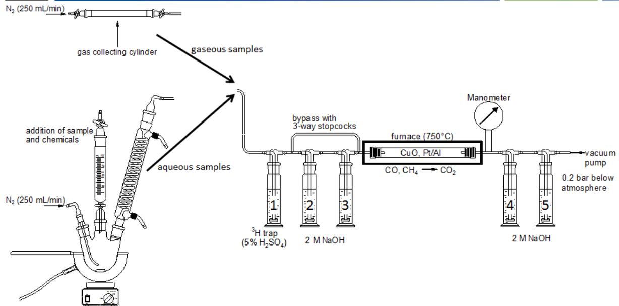
**Figure 7 Experimental design for C-14 extraction of gaseous and dissolved aliquots of experiments with Zry-4 specimens**
