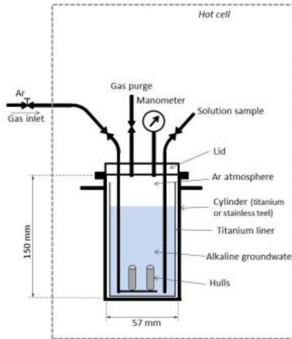
**Figure 5 : Schematic description of experimental setup for static leaching tests.**
