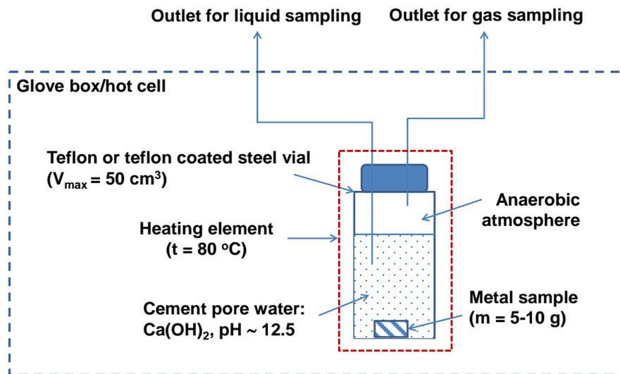
**Figure 9 : Proposed layout of the static leaching test setup in an autoclave in glove box under reducing atmosphere.**
