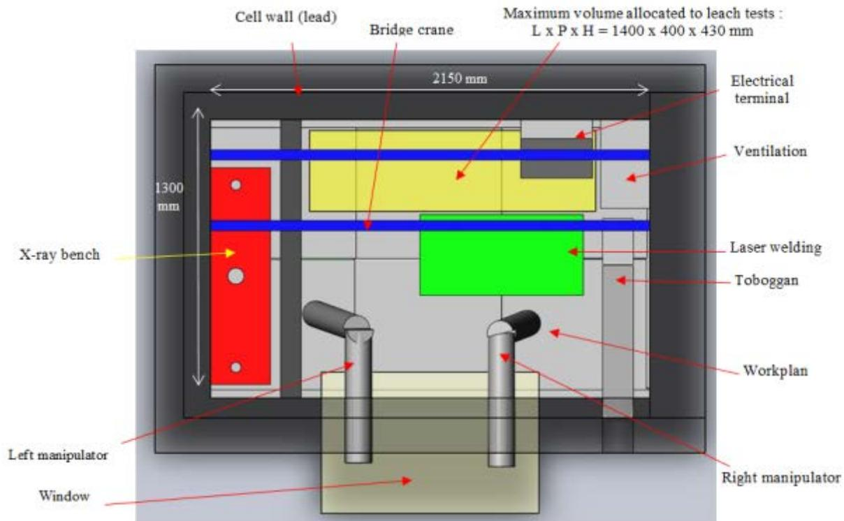
Figure 4: Schematic top view of the I1 hot cell.
