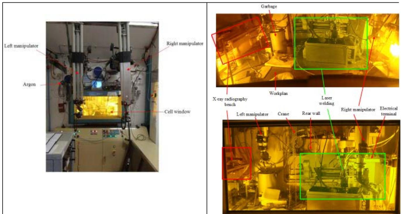
**Figure 3 : Front view and interior of the I1 hot cell.**
