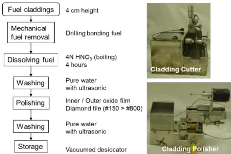
**Figure 11 : Pretreatment for specimens.**
