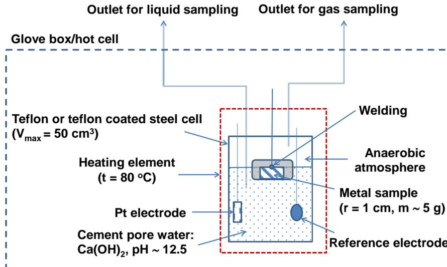
**Figure 10 : Proposed layout of the accelerated leaching test setup in an autoclave in a glove box under reducing atmosphere.**
