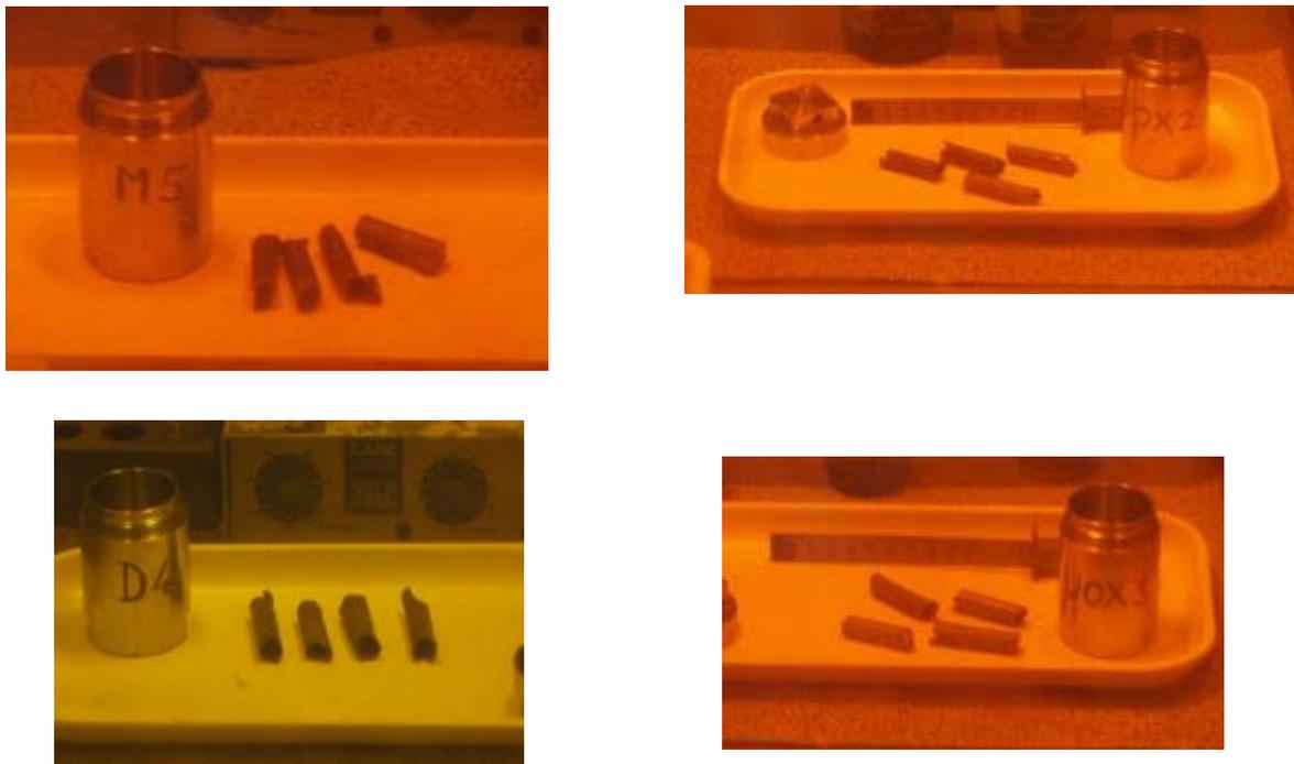
**Figure 2: Photograph (taken through a cell window) of the sheared cladding.**
