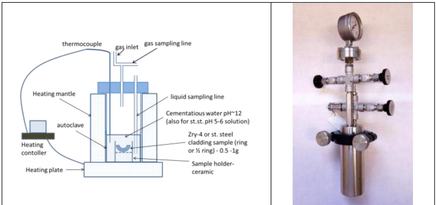
**Figure 14 : Schematic diagram of the autoclave set-up and picture of the autoclave (with Teflon lining).**
