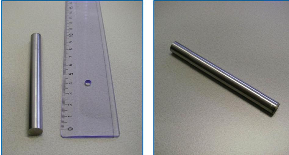
**Figure 8 : A non-irradiated Zry-4 specimen before cutting.**
