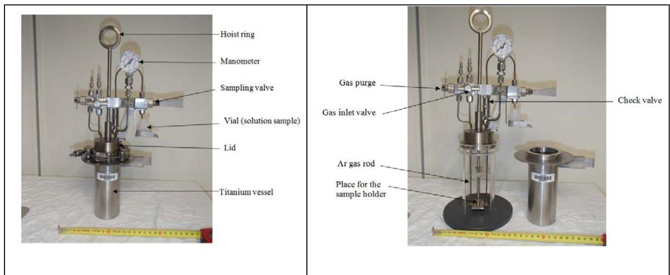
**Figure 6 : Overall view of the leaching reactor (open and closed).**
