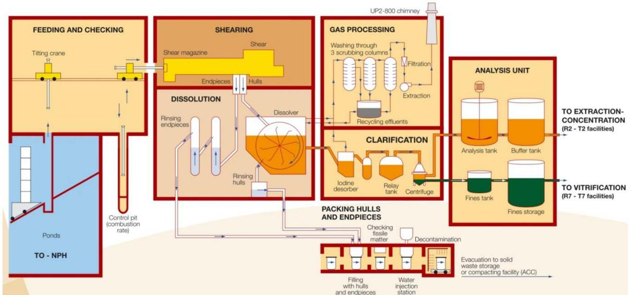
**Figure 1 : Processing of the structural waste (hulls and end-pieces) in AREVA La Hague.**
