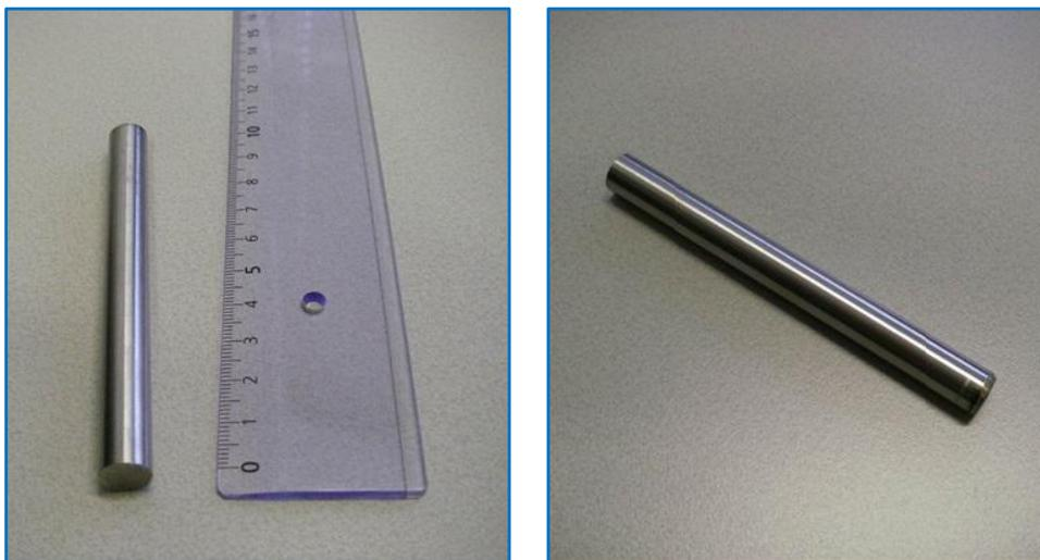
**Figure 6: A non-irradiated Zry-4 specimen before cutting.**
