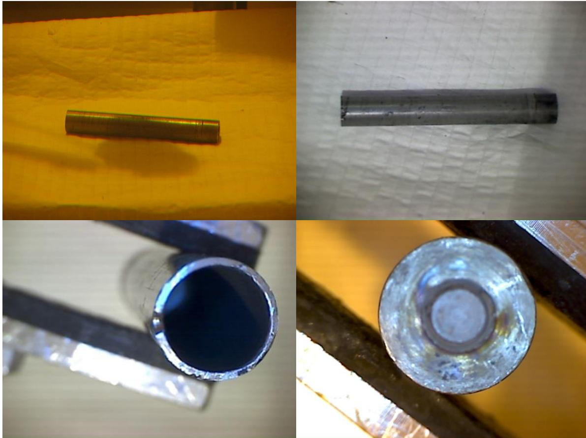
**Figure 8 Irradiated Zry-4 plenum specimen used for the dissolution experiments**
