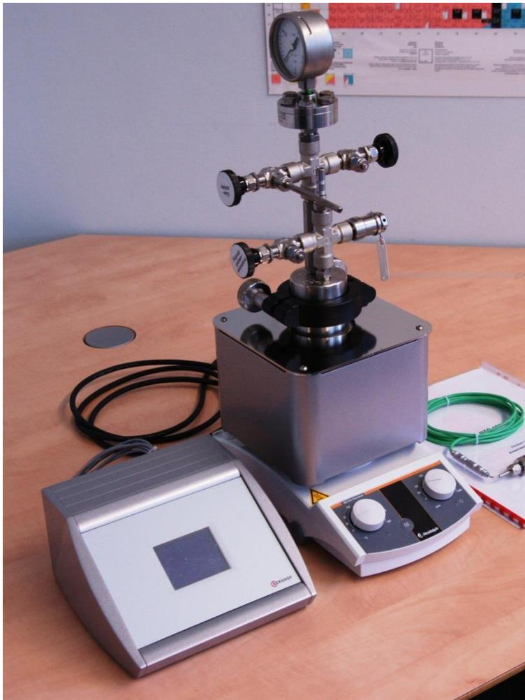
**Figure 7 Autoclave with heating mantle and hot plate for assuring a constant temperature during the leach tests**
