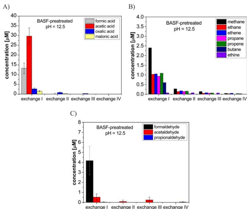
**Figure 9.3: Concentrations of carboxylic acids (a), gaseous hydrocarbons (b) and aldehydes (c) as a function of solution replacements (pH = 12.5)**
