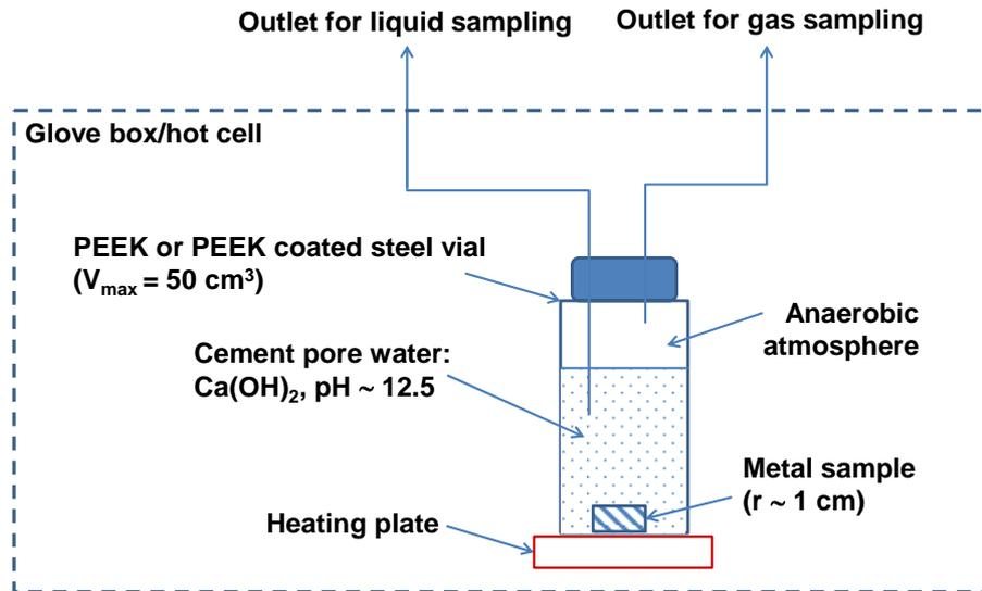
Figure 11.2: Proposed layout of the static leaching test setup in glove box/hot cell under reducing atmosphere
