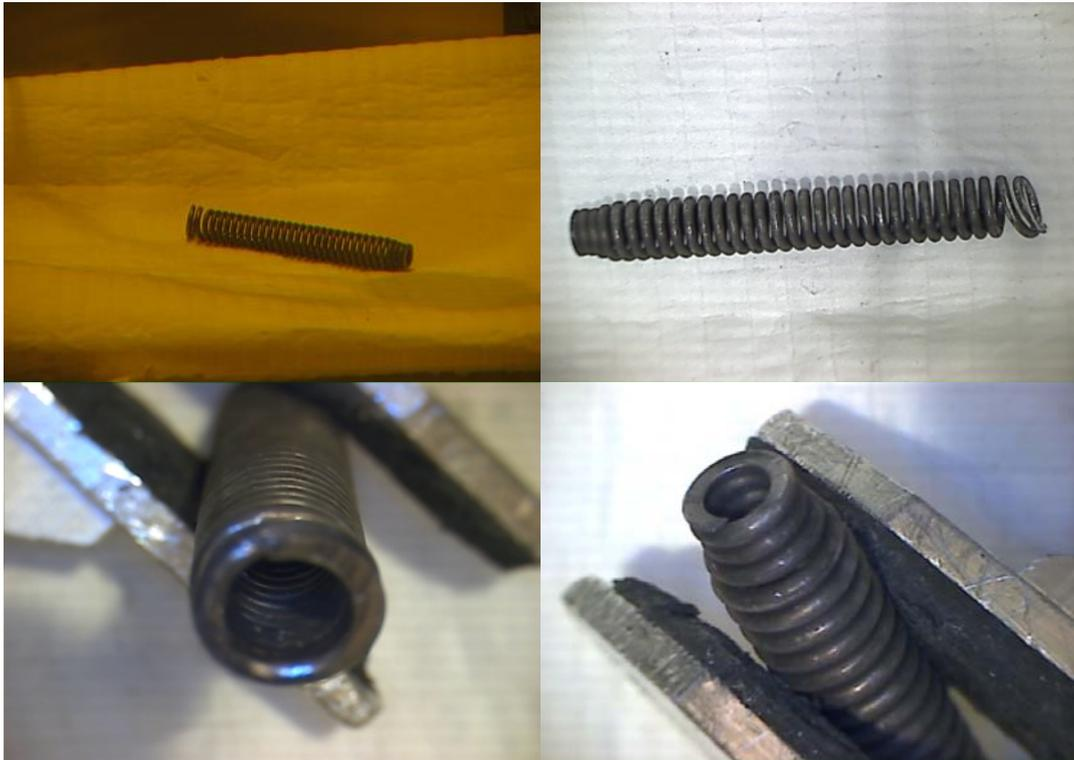
**Figure 7.1: Irradiated stainless steel plenum spring used for the dissolution experiments**
