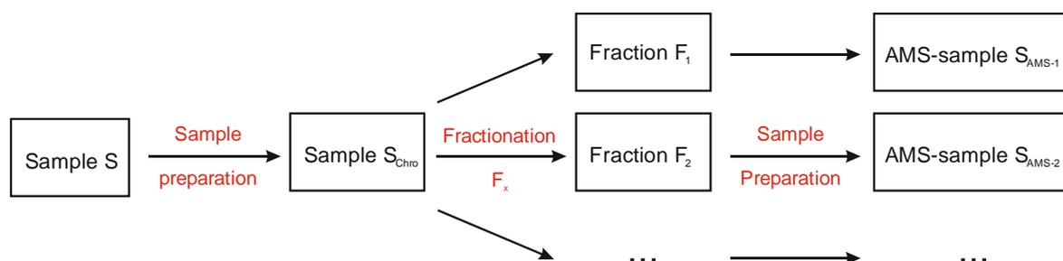
**Figure 9.4:** Simplified flow chart of the chromatographic separation of  $^{14}\text{C}$  bearing organic compounds coupled to  $^{14}\text{C}$  detection by AMS
