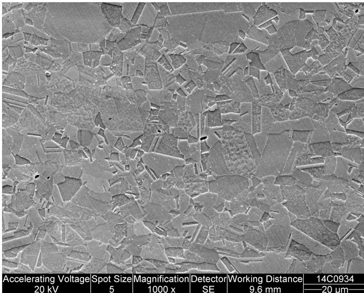
**Figure 12.1: SEM picture of the surface microstructures of Loviisa steel**
