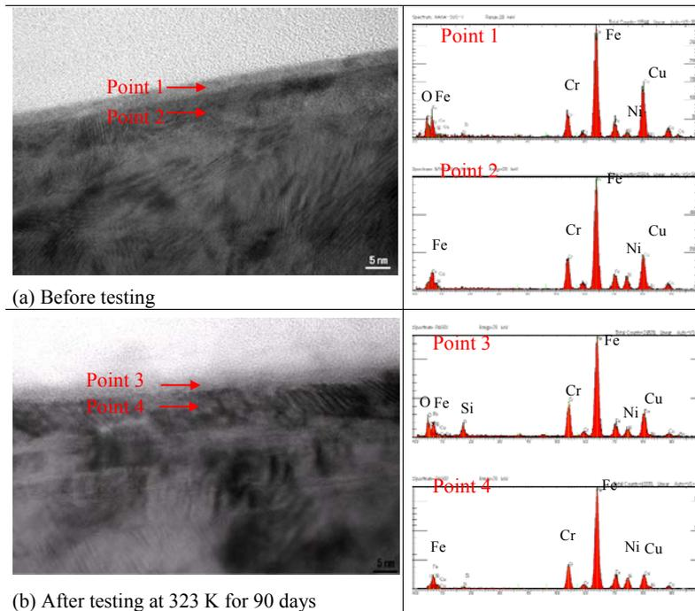
**Figure 10.7: TEM and EDX spectra of surface layer**
