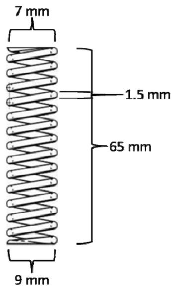
**Figure 7.2: Scheme of the stainless steel plenum spring with dimensions**
