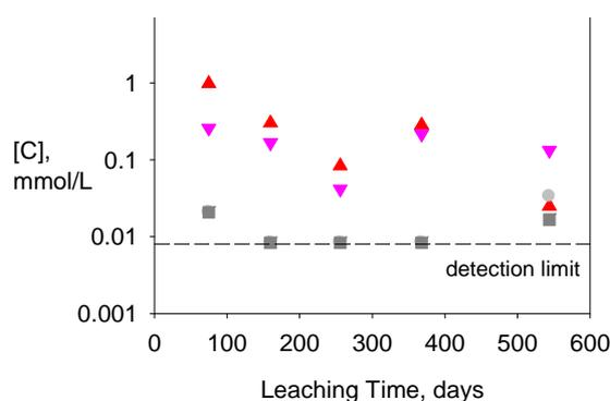
**Figure 12.4a: Dissolved organic (red and pink) and dissolved inorganic (grey) carbon in the preliminary leaching tests of Loviisa steel in groundwater at pH 8.5 as a function of leaching time**
