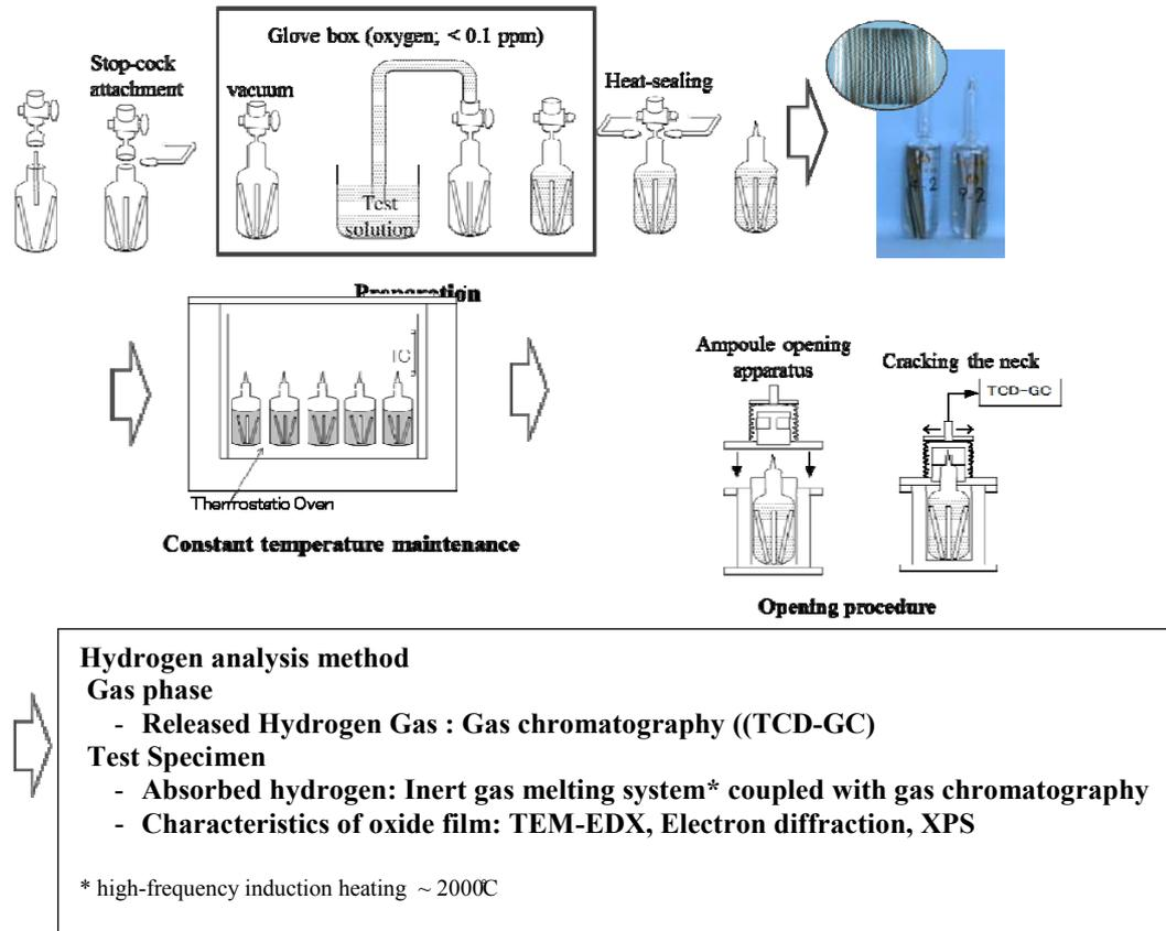
**Figure 10.2: Corrosion test and hydrogen measurement procedure of SS**
