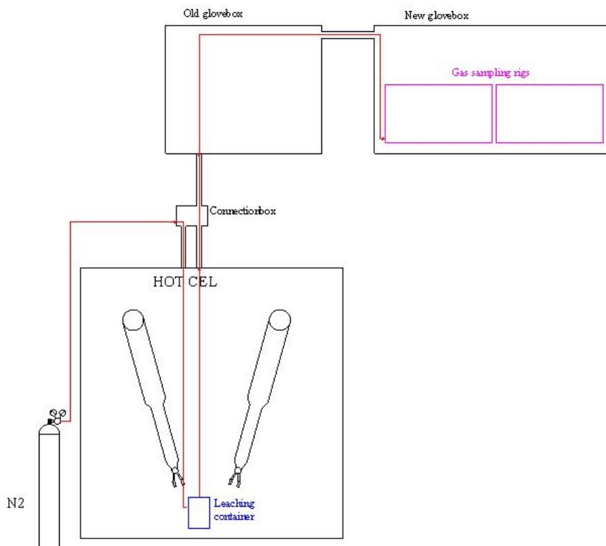
Figure 8.4: Schematic drawing of the leaching experiment in the G1 cell in the HCL
