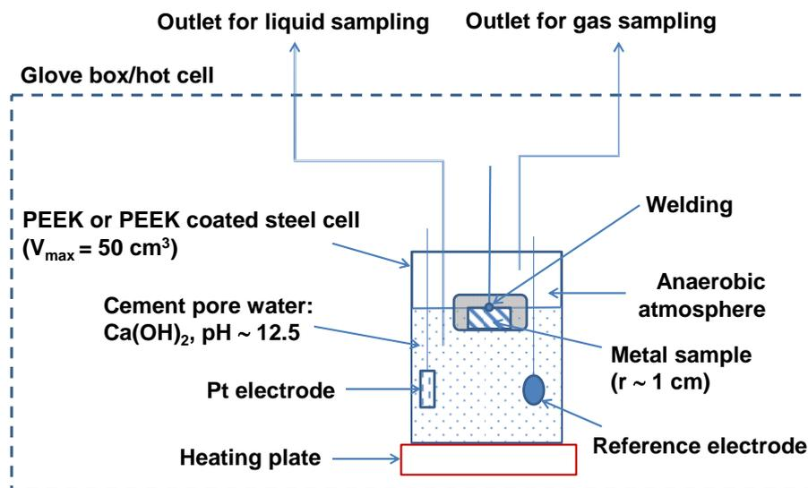
Figure 11.3: Proposed layout of the accelerated leaching test setup in glove box/hot cell under reducing atmosphere
