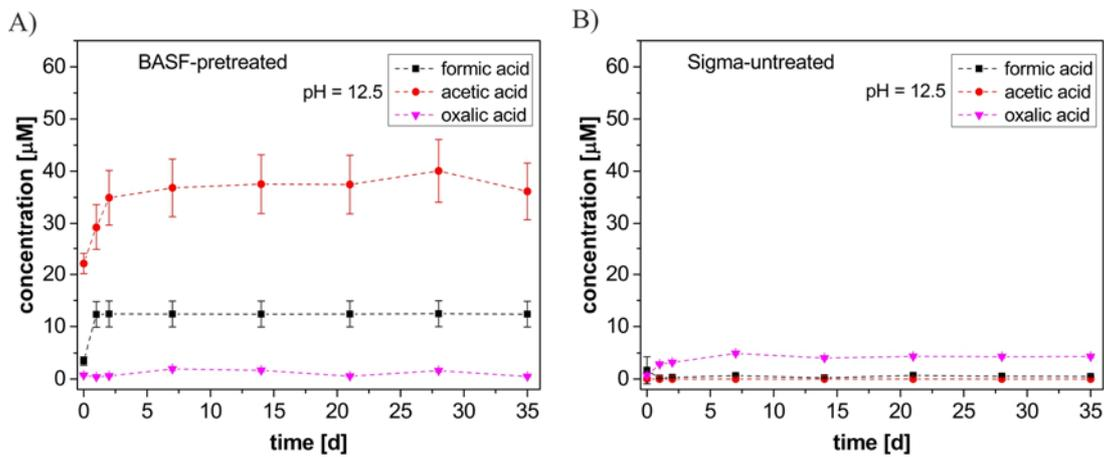
**Figure 9.1: Time dependence of the concentrations of carboxylic acids during the anoxic corrosion of two different iron powders at pH = 12.5**
