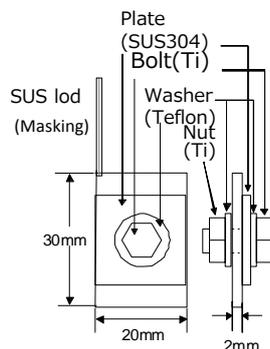
**Figure 10.3: Test specimen for measurement of repassivation potential for crevice corrosion ( $E_{\text{R,CREV}}$ )**
