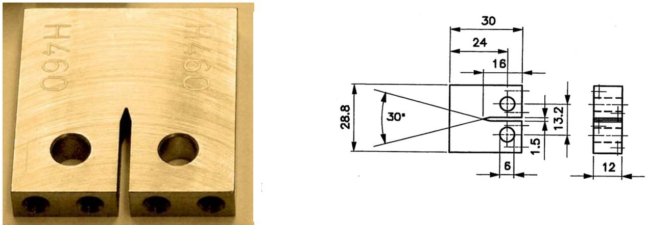
**Figure 8.5: CT specimen photo (left) and technical drawing (right)**
