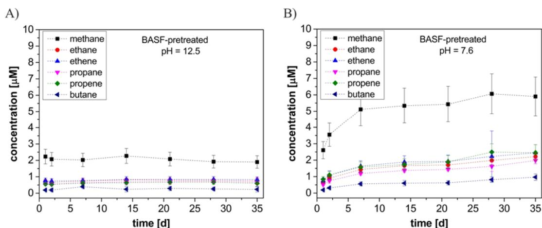
**Figure 9.2: Time dependence of the hydrocarbon concentrations during the anoxic corrosion of pre-treated BASF iron powder at pH = 12.5 (A) and pH = 7.6 (B)**
