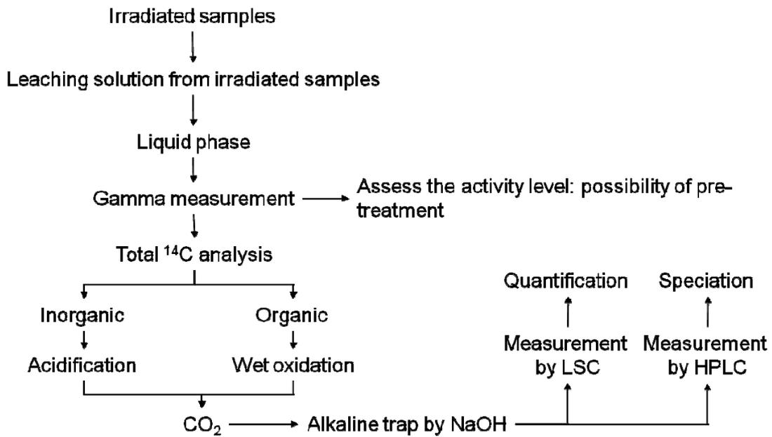
Figure 3.2: Experimental setup for the determination of Carbon-14 species
