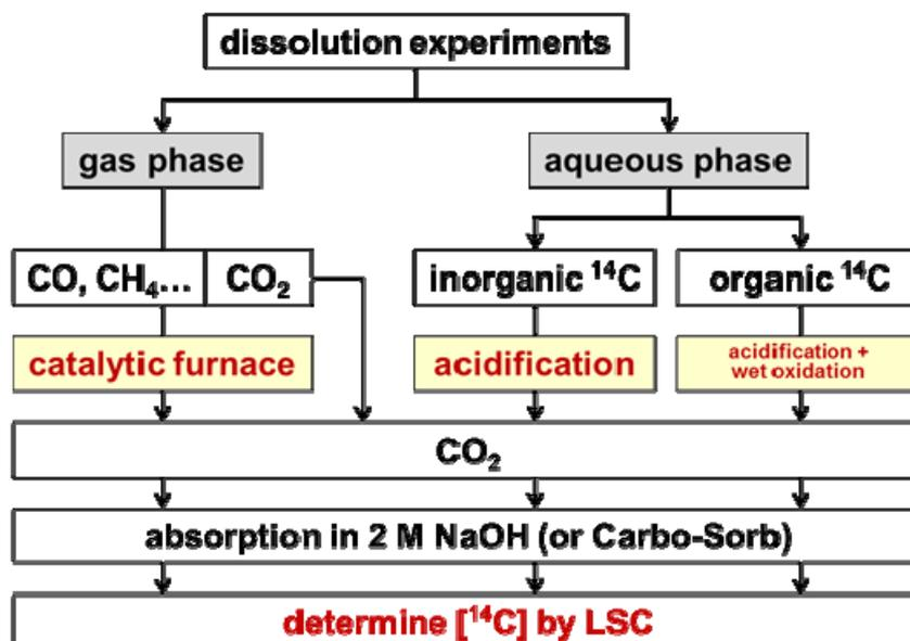
**Figure 7.4: Scheme of  $^{14}\text{C}$  extraction procedure for gaseous and dissolved aliquots of experiments with stainless steel specimens**
