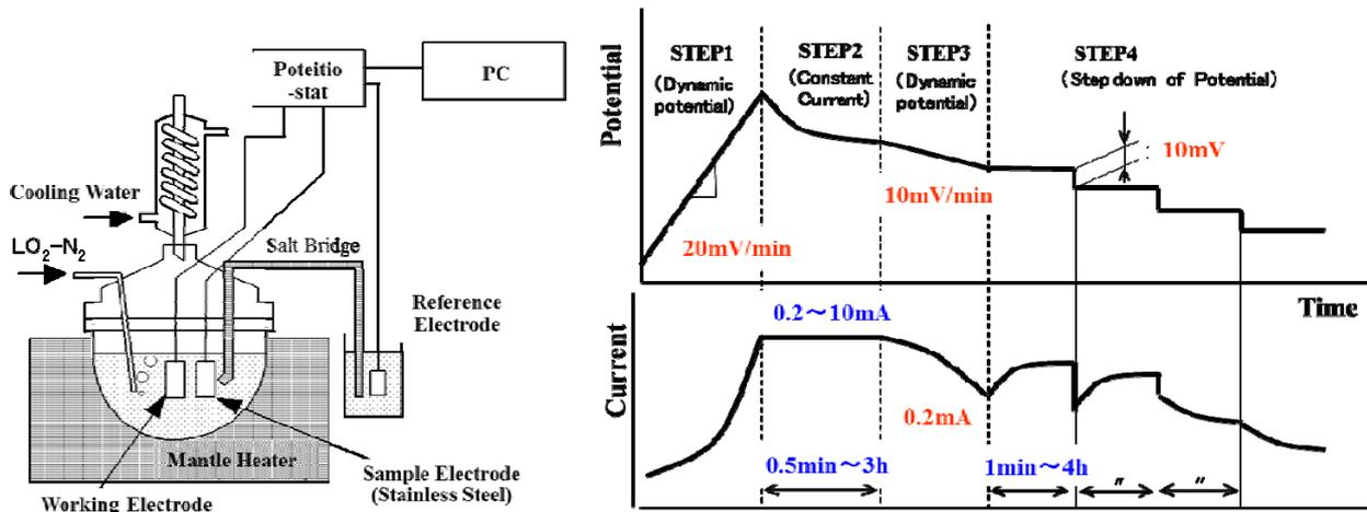
Figure 10.4: Apparatus and measurement method of repassivation potential for crevice corrosion ( $E_{R,CREV}$ )
