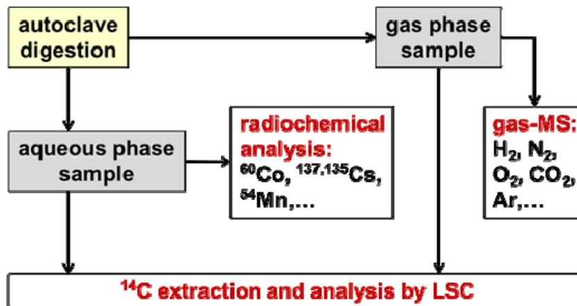
**Figure 7.3: Scheme of the experimental procedure for quantification of  $^{14}\text{C}$  species of stainless steel specimens**
