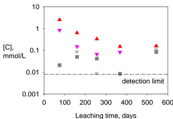
**Figure 12.4b: Dissolved organic (red and pink) and dissolved inorganic (grey) carbon in the preliminary leaching tests of High carbon steel in groundwater at pH 8.5 as a function of leaching time**
