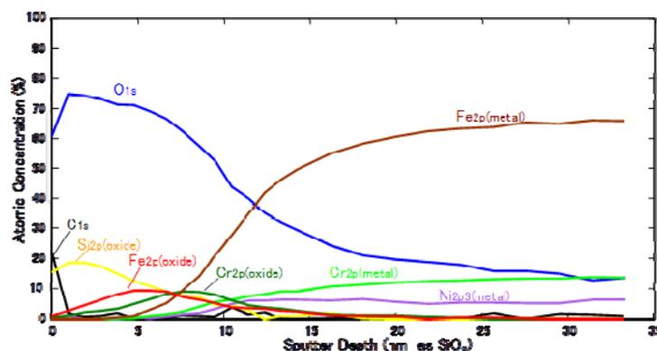
**Figure 10.8: Depth profile of SS surface layer after 90-day test through XPS analysis**
