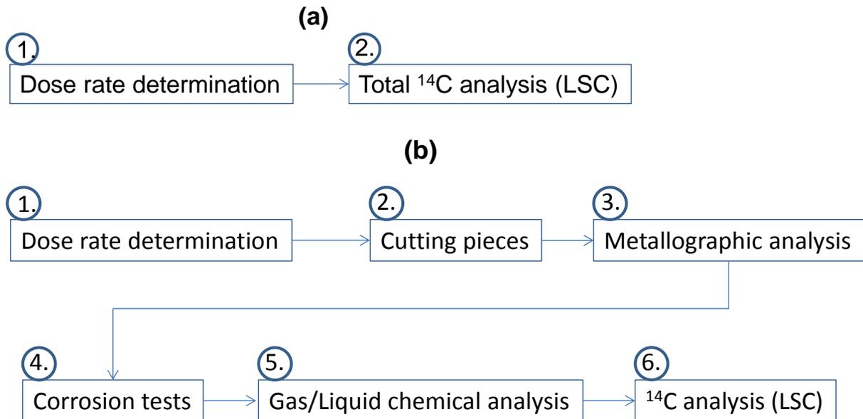
**Figure 11.4: Proposed sequence of the total  $^{14}\text{C}$  analysis (a) and the corrosion test followed by carbon speciation analysis (b)**
