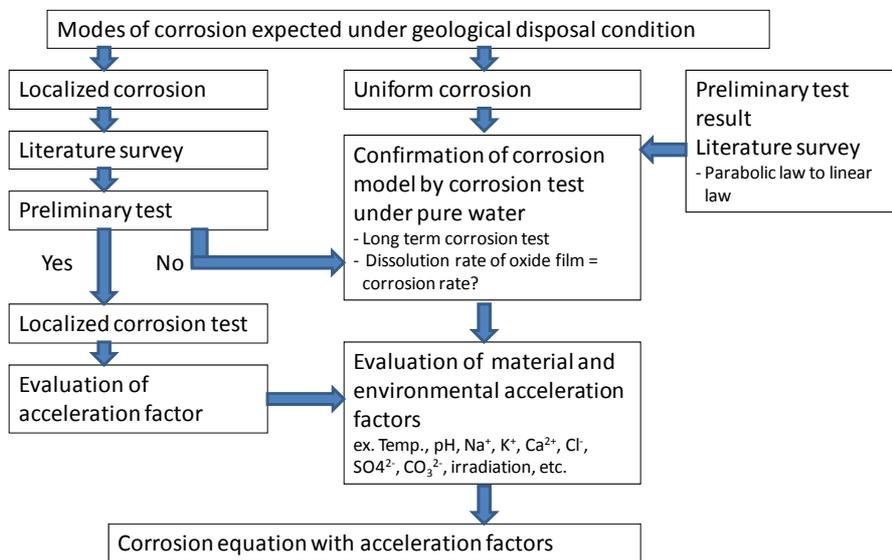
**Figure 10.1: Method to evaluate corrosion expected under geological disposal condition**
