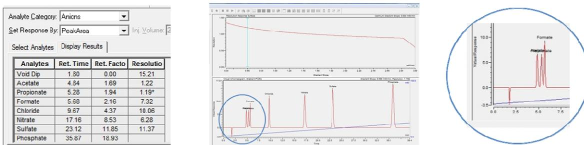
**Figure 4.3: Carboxylic acids Chromatogram**
