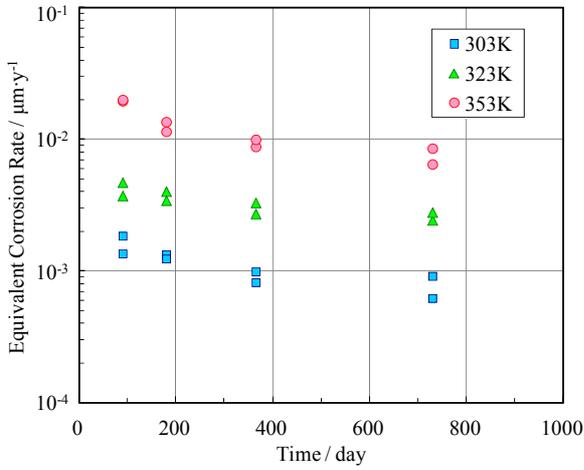
**Figure 10.5: Equivalent SS corrosion rate thickness**
