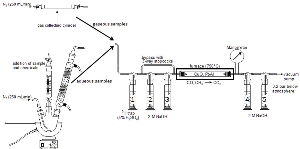
**Figure 7.5: Experimental design for  $^{14}\text{C}$  extraction of gaseous and dissolved aliquots of experiments with stainless steel specimens**
