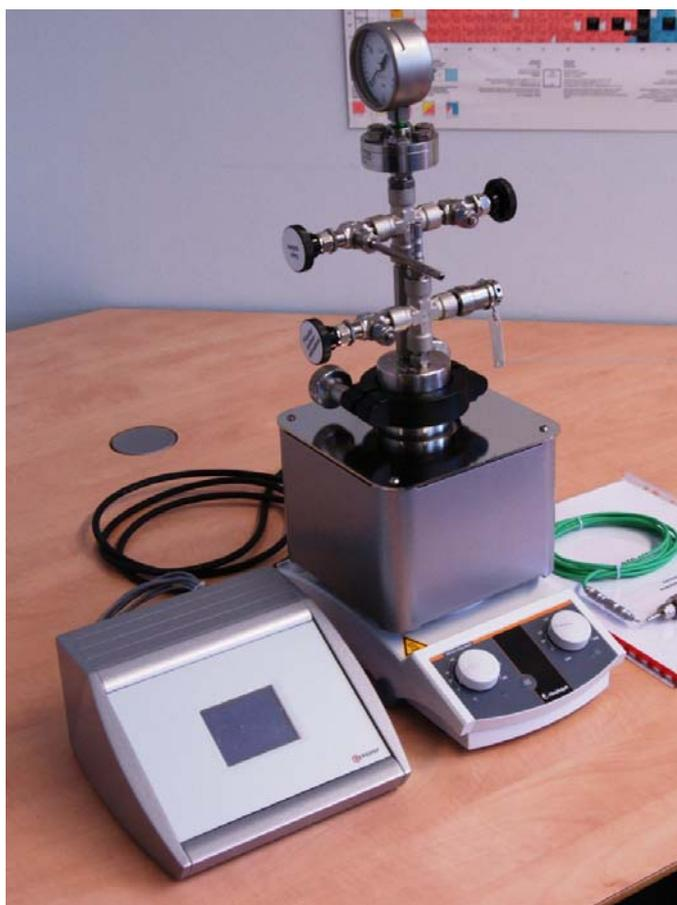
**Figure 6.1: Autoclave with heating mantle and hot plate for assuring a constant temperature during the leach tests**
