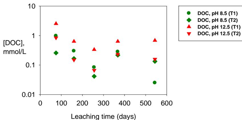
**Figure 12.3: Dissolved organic carbon (DOC) in the preliminary leaching tests of Loviisa steel in simulated groundwater at pH 8.5 and 12.5 as a function of leaching time. T1 represents tests with  $m/V=50$  g/100 mL and T2 tests with  $m/V=25$  g/100 mL**
