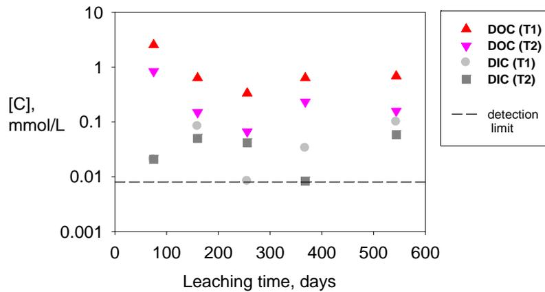
**Figure 12.2: Dissolved inorganic (DIC) and organic (DOC) carbon in the preliminary leaching tests of Loviisa steel in simulated groundwater at pH 12.5 as a function of leaching time. T1 represents tests with  $m/V=50$  g/100 mL and T2 tests with  $m/V=25$  g/100 mL**
