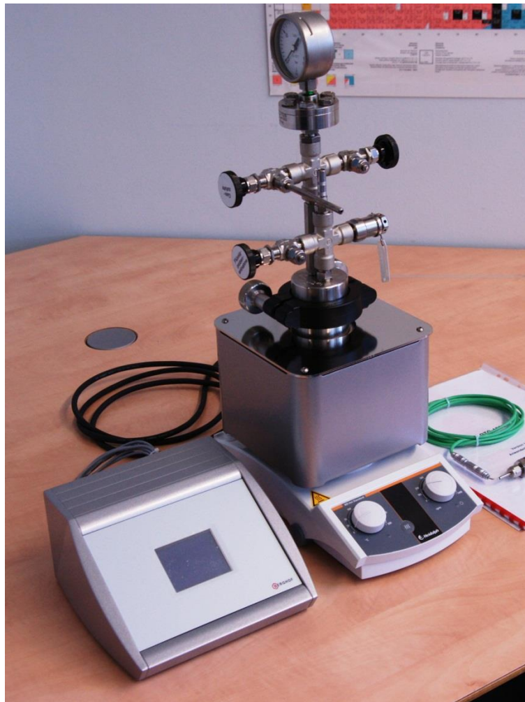
Figure 1: Autoclave with heating mantle and hot plate for assuring a constant temperature during the leach tests
