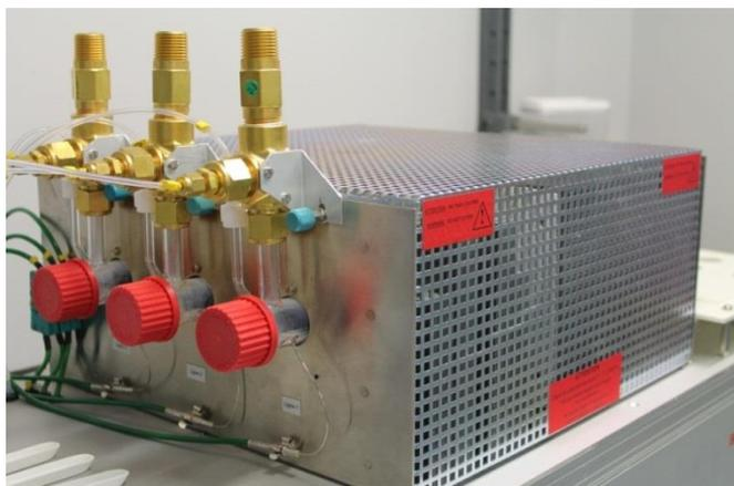
Figure 3: Tri-tube pyrolysis furnace.
