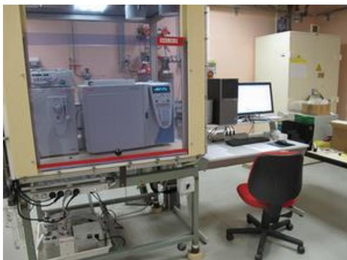
Figure 8: Gas chromatography-coupled with mass spectrometry.
