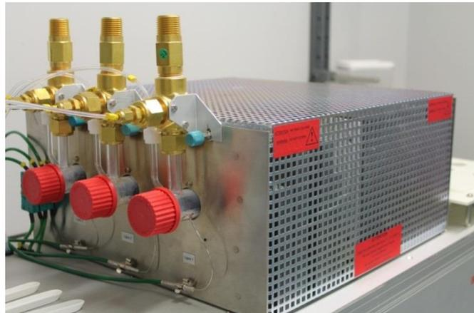
Figure 3: Tri-tube pyrolysis furnace.
