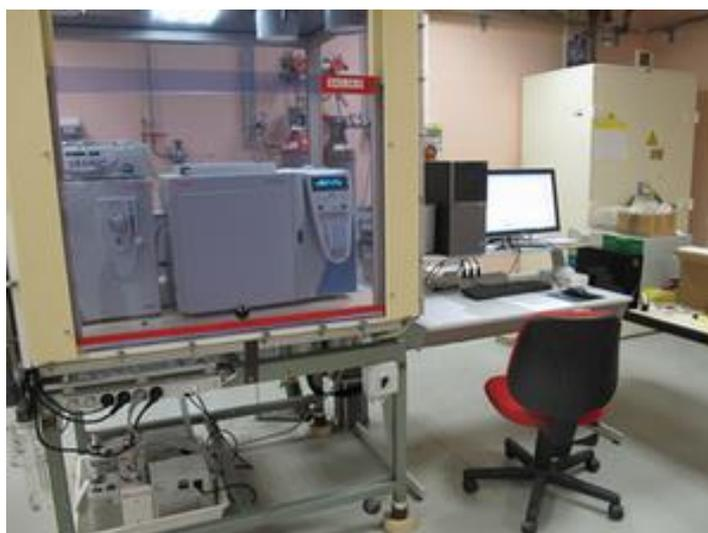
Figure 8: Gas chromatography-coupled with mass spectrometry.
