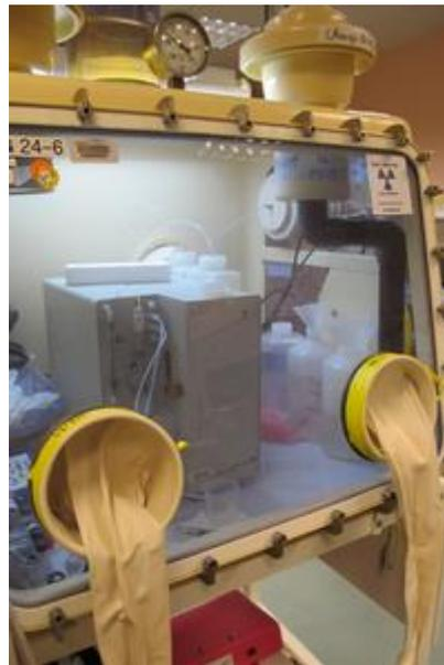
Figure 2: TOC analyser in a glove box.
