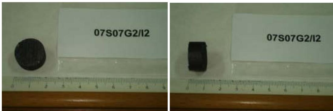
**Figure 2.6.1 - One of the i-Graphite samples from Latina NPP**
