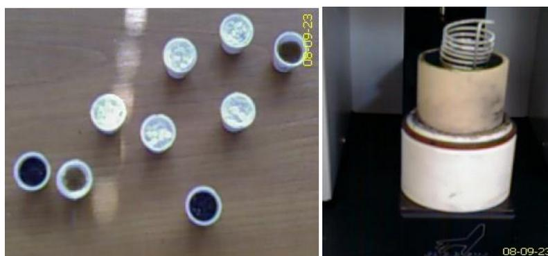
**Figure 16. The combusto-cones prepared for the resin combustion (left) and the combustion system (right).**
