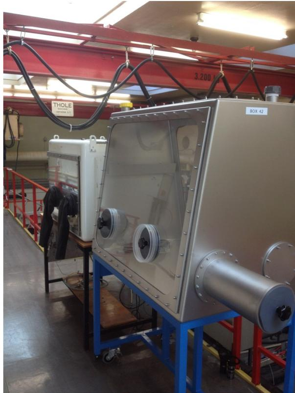
**Figure 8.3: A glove box to be used for placing of RCD rig, installed above the chemical cell**
