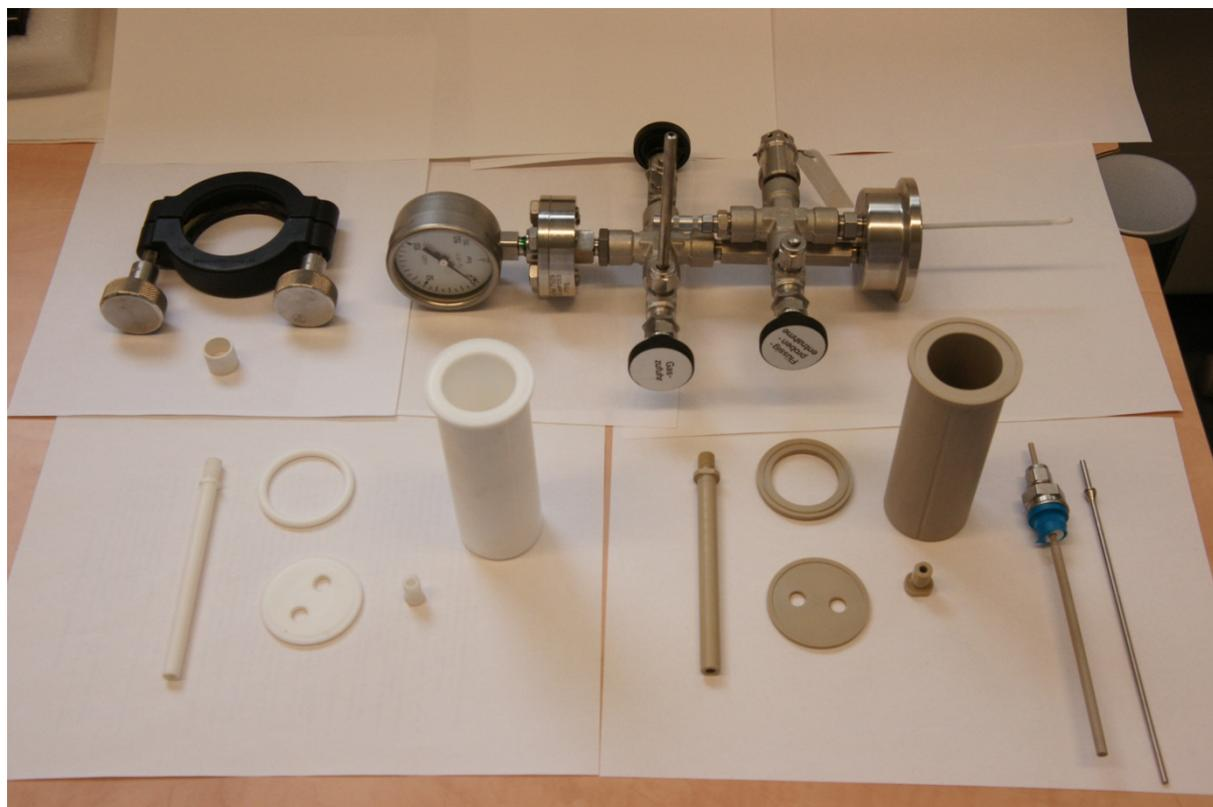
**Figure 6.1: Autoclave with old Teflon (left) and new PEEK linings (right). The autoclave will be used with the more stable PEEK lining. The cladding samples will be placed in small PEEK crucibles with holes to allow the water to drain from the sample.**
