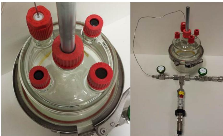
**Figure 11.1: Glass cell for accelerated corrosion test setup**
