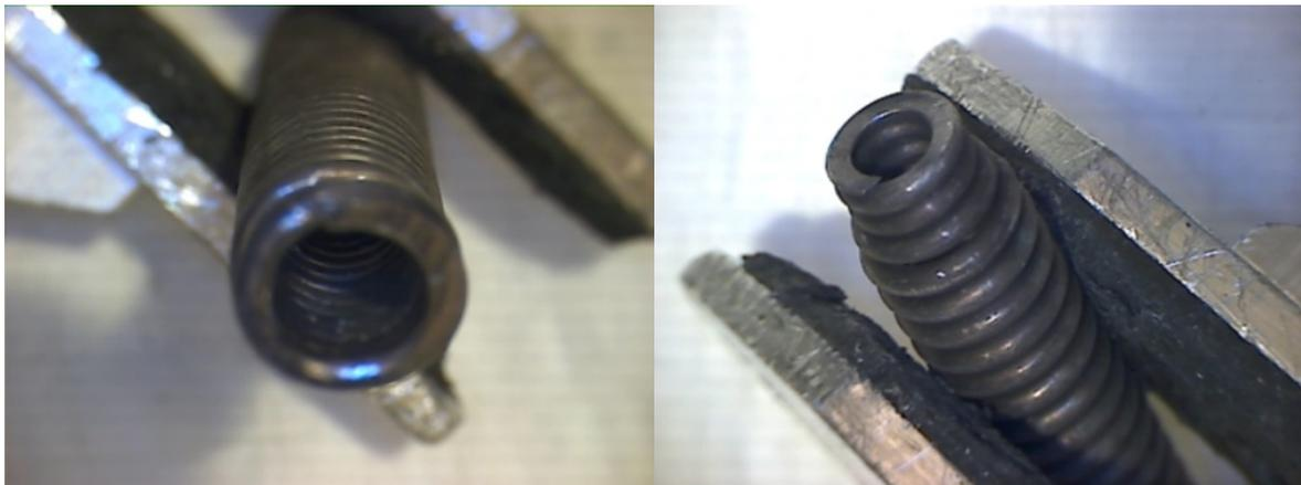
**Figure 7.2: Photos of the irradiated stainless steel plenum spring.**
