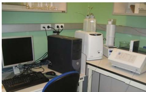
**Figure 4.3: Gas Chromatograph coupled to a Mass Spectrometer (left) and Ion Chromatography system (right)**
