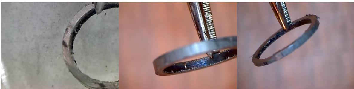
**Figure 16: Black/blueish precipitates seen on the inner surface of the irradiated Zircaloy-4 cladding.**
