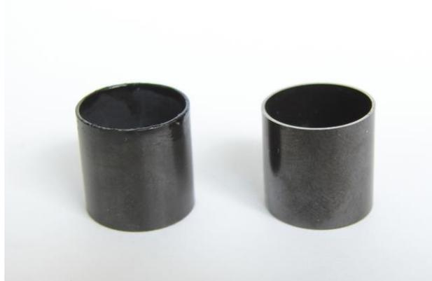
**Figure 19** Oxidised Zy-4 tube cut and painted at the end (left) and oxidised Zy-4 tube cut (right)
