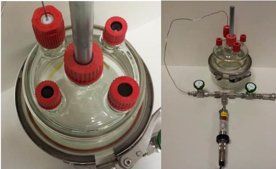
**Figure 29 Glass cell for accelerated corrosion test setup.**
