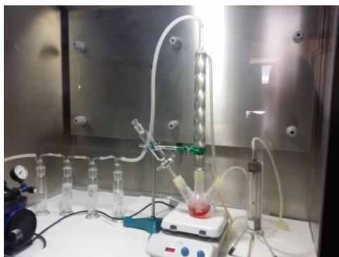
**Figure 21** Experimental set-up for C-14 measurements in irradiated Zy-4.
