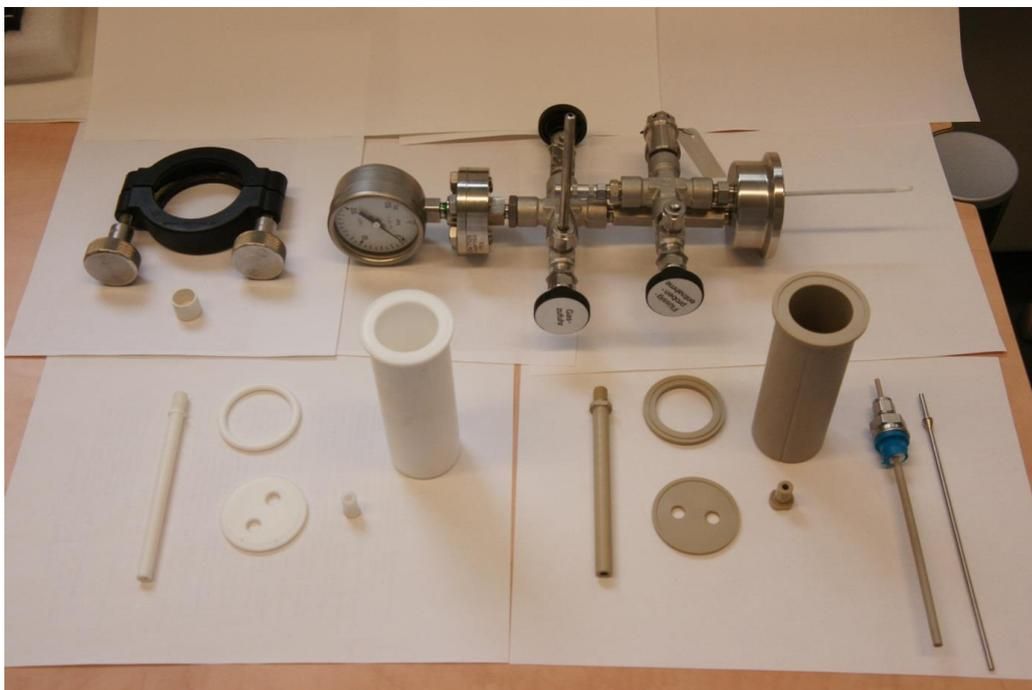
**Figure 9** Autoclave with old Teflon (left) and new PEEK (right) linings. The autoclave will be used with the more stable PEEK lining in small PEEK crucibles with holes to allow the water to drain from the sample.
