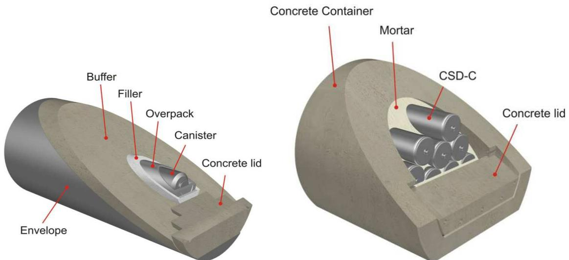
Figure 2. Example of a supercontainer and a monolith design for vitrified HLW canisters and compacted waste ('CSD-C'), respectively.
