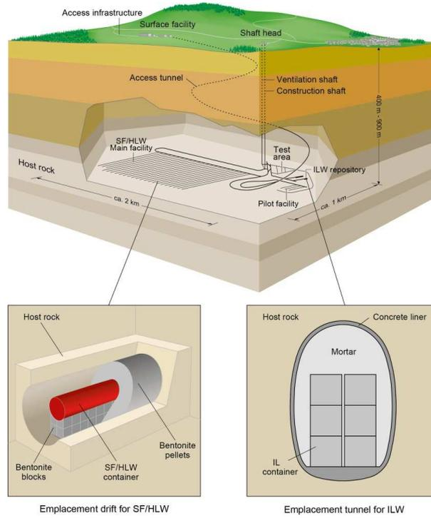
**Figure 1. Conceptual outline of a deep geological repository for SF/HLW and ILW (NAGRA 2008b, modified)**
