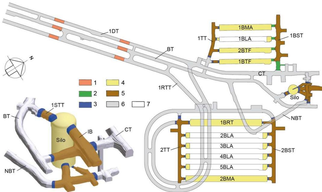
**Figure 1-2.** Overview of SFR after closure with detailed view of silo. Key to colors. 1 Tunnel plugs, 2. Transition material, 3. Mechanical plugs of concrete, 4. Backfill material made of MacAdam, 5. Low hydraulic conducting section made of bentonite, Tunnel backfill material of MacAdam, 7. Non backfilled waste vaults
