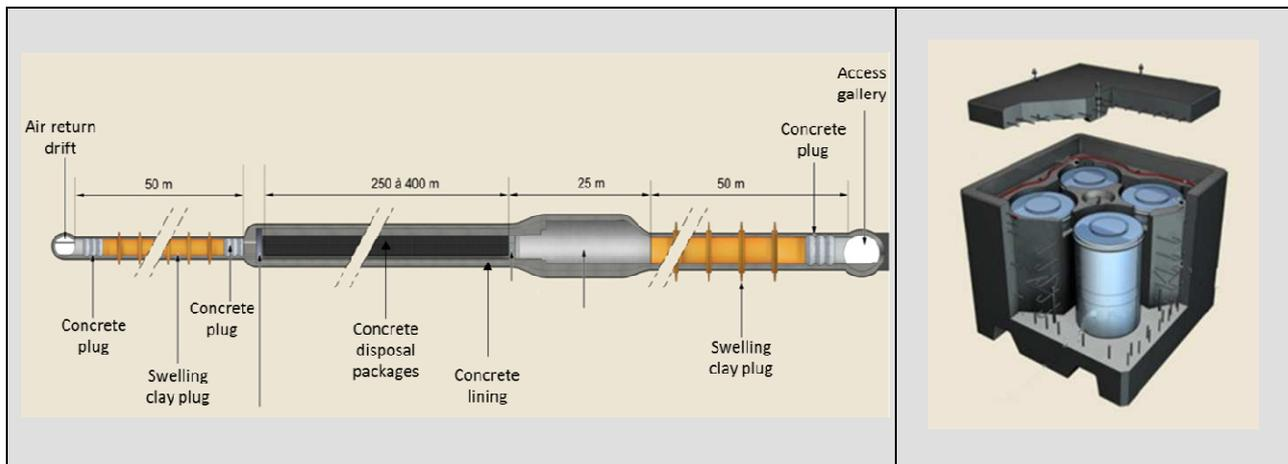
**Figure 4: Schematic illustration for IL-LL waste disposal cell (left) and IL-LL waste disposal package (right)**
