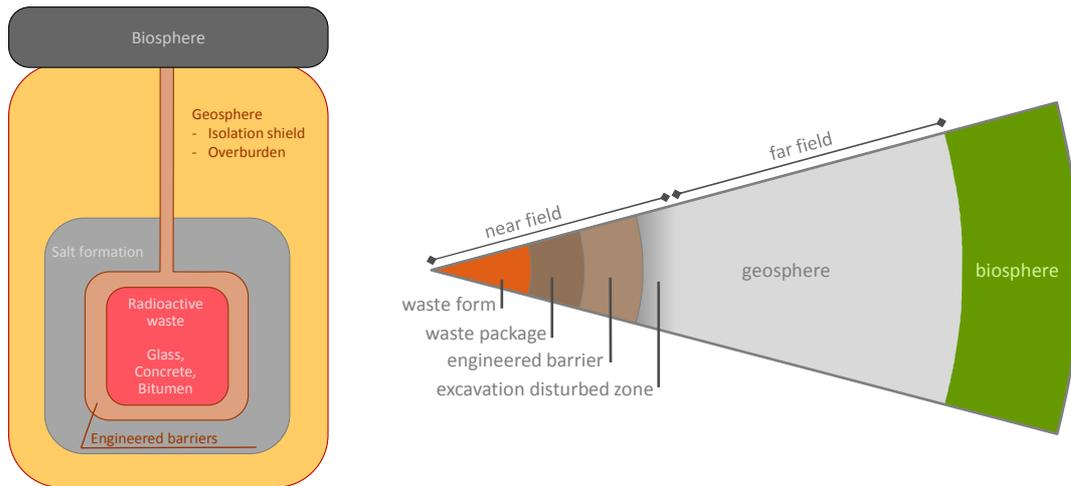
**Figure 4. Principle of a multi-barrier system in salt formations (left), and in Boom Clay (OPERA, right)**
