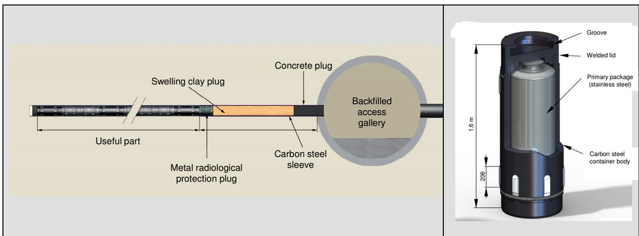
**Figure 3: Schematic illustration of the design for HL waste disposal cell (left) and HL waste package (right)**
