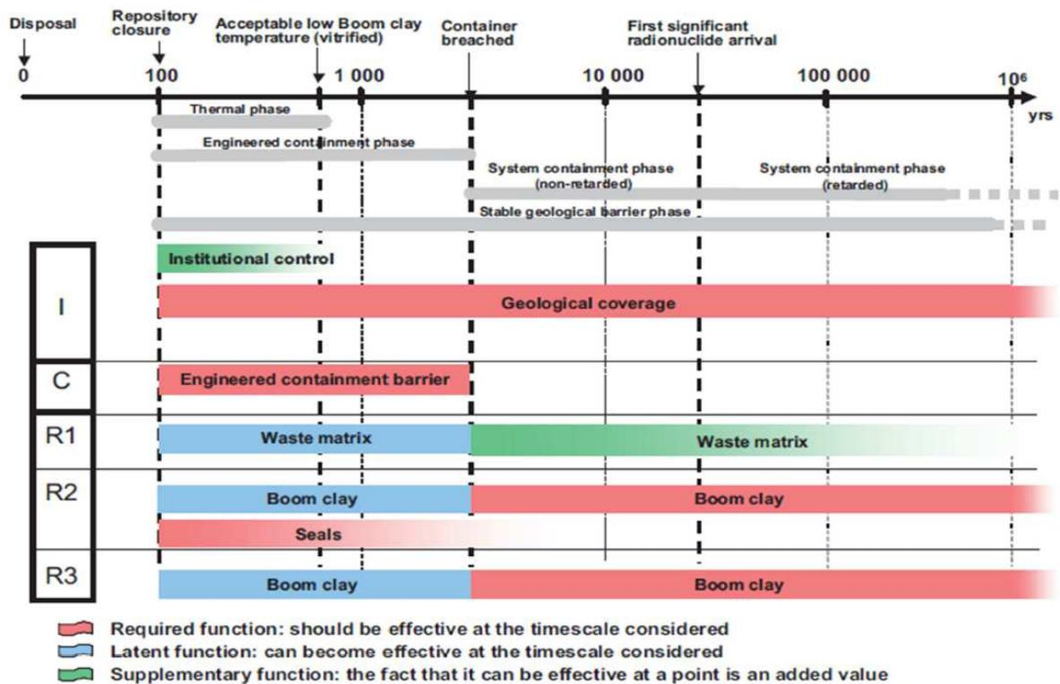
Figure 2 Relationship between safety functions and time for the disposal of spent fuel and high level waste. I = Isolation, C = Containment, R= retardation (time periods are illustrative) [IAEA, 2011].
