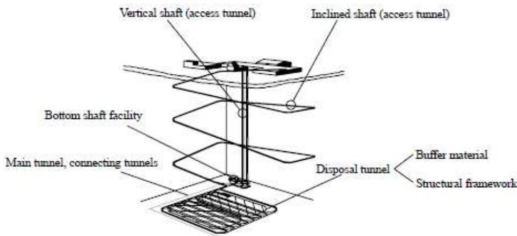
**Figure 2: Basic concept for the TRU repository in Japan.**
