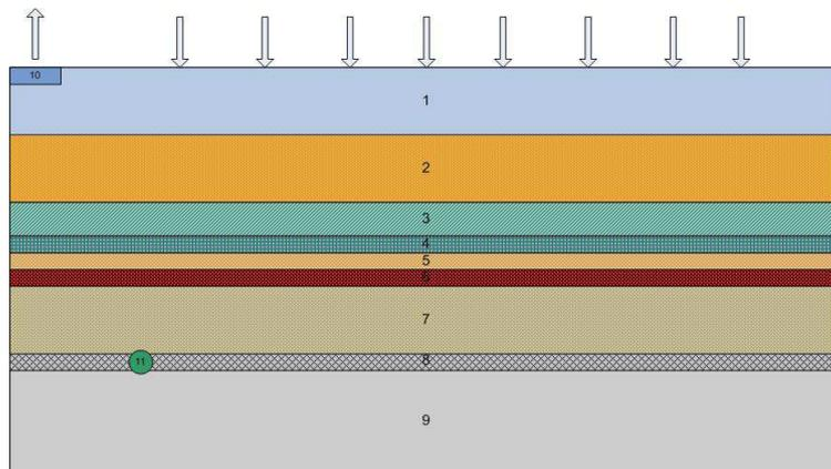
**Figure 4: Far field model (1 – glacial loam, 2 – sand, 3 – anhydrite, 4 – limestone, 5 – sandstone, 6 – clay, 7 – sandstone, 8 – weathered crystalline rocks, 9 – monolithic crystalline rocks, 10 – groundwater discharge area, 11 – radionuclide flux from the crystalline rock)**
