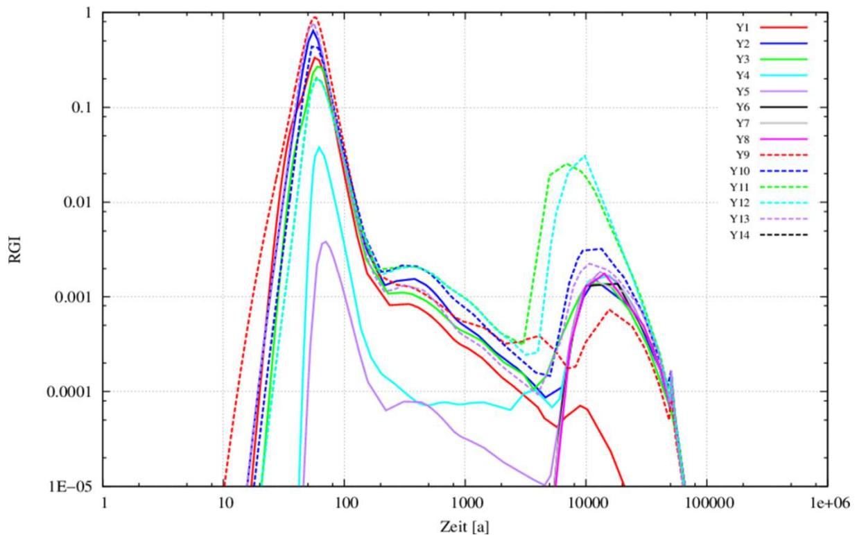
**Figure 3: RGI resulting from the C-14 flux out of the spent fuel containers calculated at the isolating rock zone boundary for different variants [Larue et al. 2013]**
