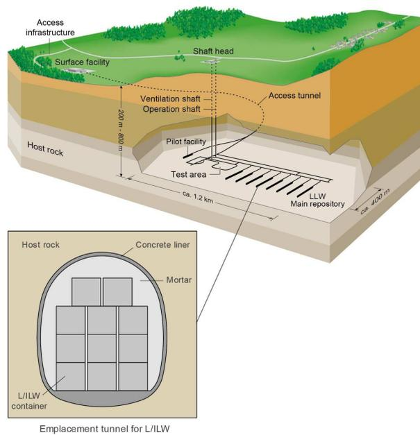
**Figure 2. Conceptual outline of a deep geological repository for L/ILW (NAGRA 2008b, modified)**
