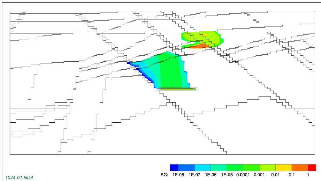
**Figure 4 Contour plot of gas saturation at 240 years post-closure for gas migration from a GDF in a higher strength rock [17].**
