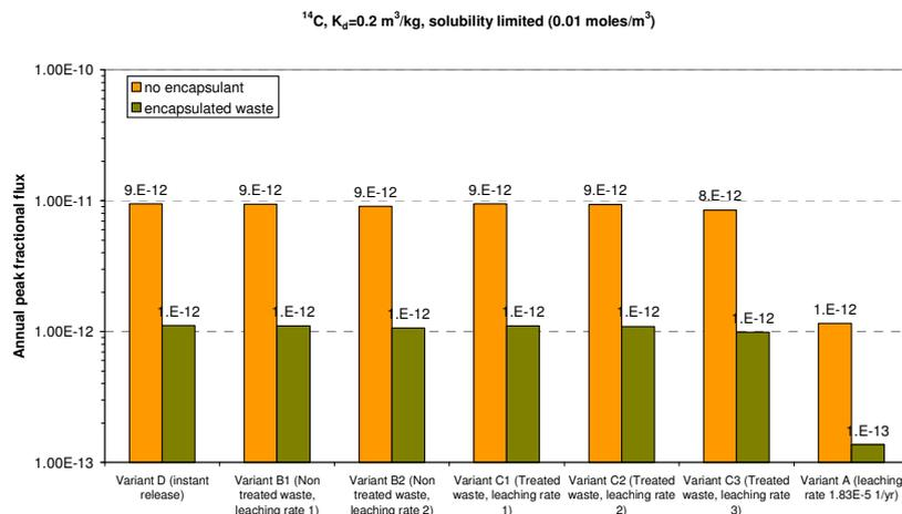
**Figure 6: Comparison of peak release for not encapsulated and encapsulated waste (results of Case 3, considering sorption and solubility limitation)**
