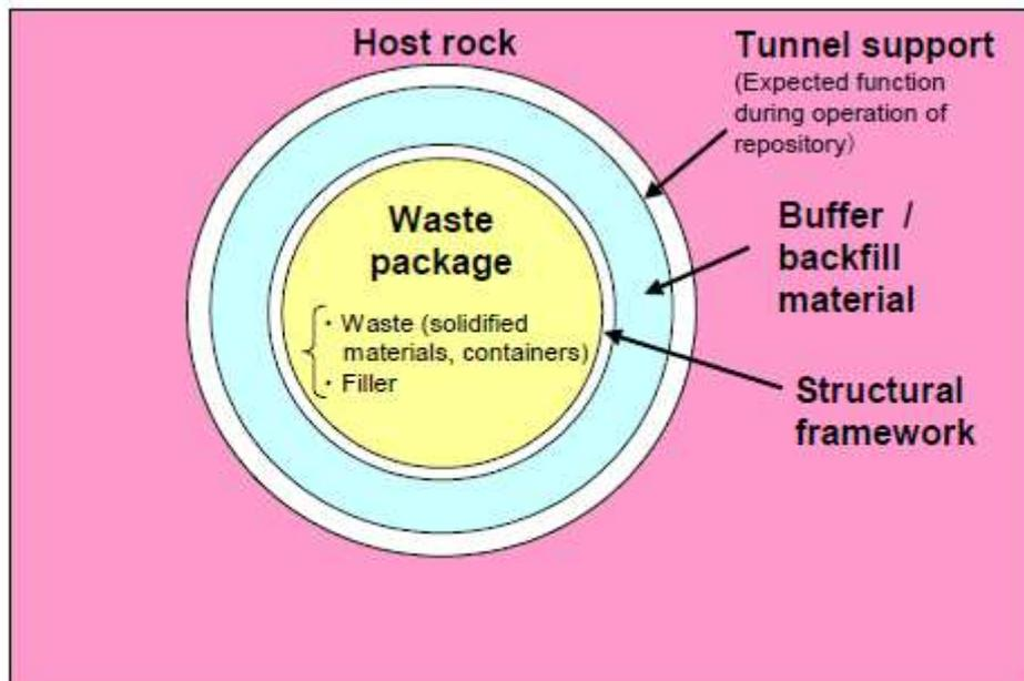
Figure 6: Basic concept for the engineered barrier system.
