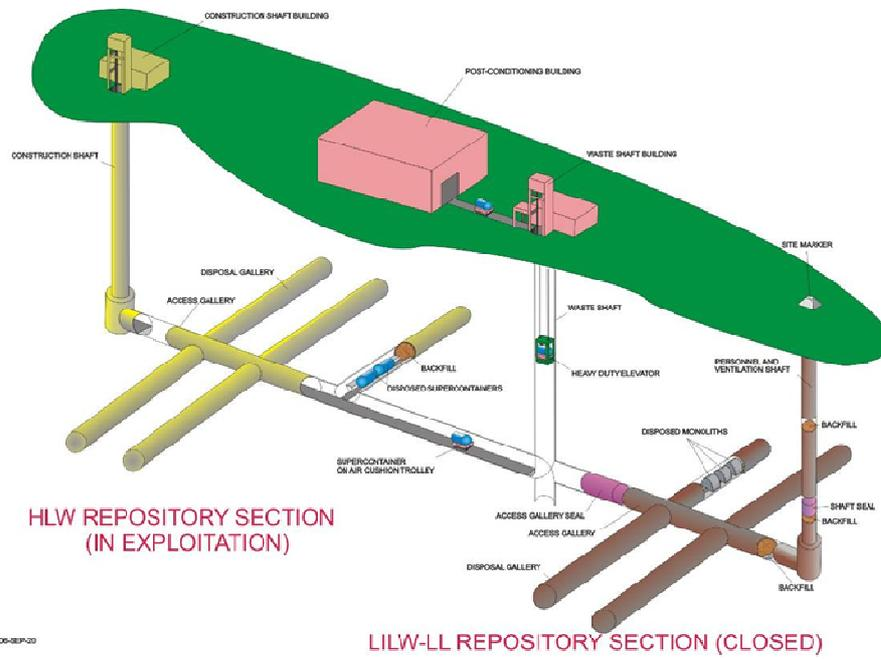
Figure 1 Reference design for the disposal of category B and C waste in Belgium
