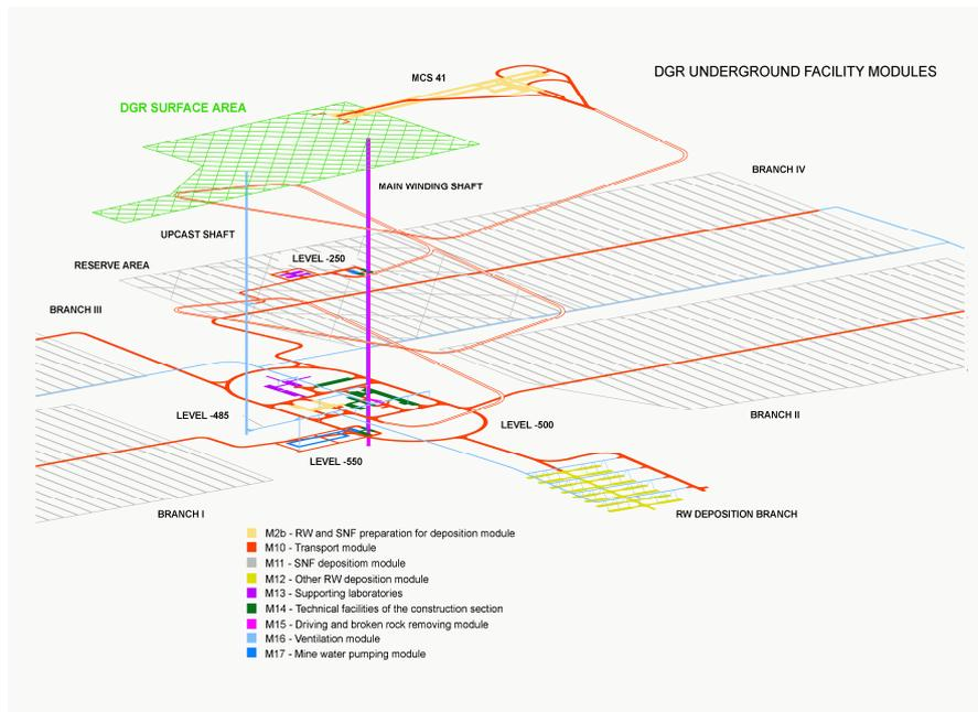
**Figure 2: Scheme of the future Czech DGR for spent fuel assemblies and ILW**
