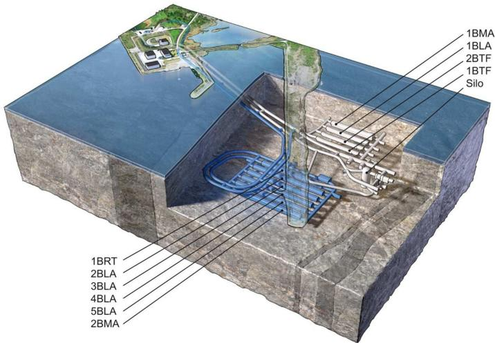
**Figure 1-1.** Schematic illustration of SFR. The grey part is the existing repository (SFR 1) and the blue part is the planned extension (SFR 3). (The waste vaults in the figure are Silo for intermediate-level waste, 1-2BMA vaults for intermediate-level waste. 1-2BTF vaults for dewatered spent ion exchange resins and incineration ashes. 1-5BLA vaults for low-level waste and BRT vault for reactor pressure vessels).
