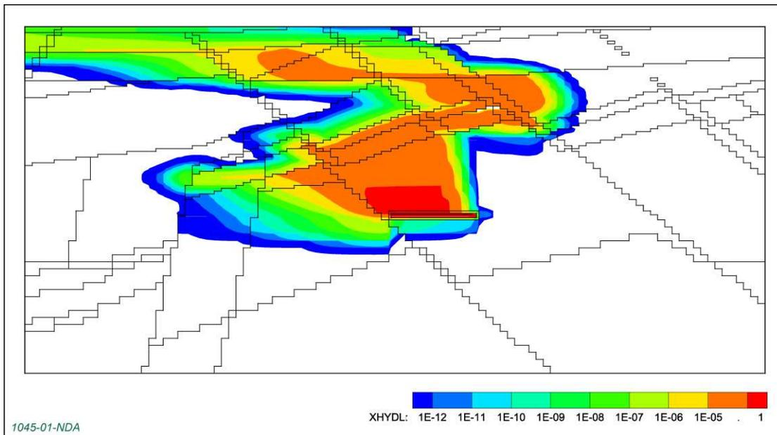
**Figure 5 Contour plot of mass fraction of dissolved gas at 240 years post-closure for gas migration from a GDF in a higher strength rock [17].**
