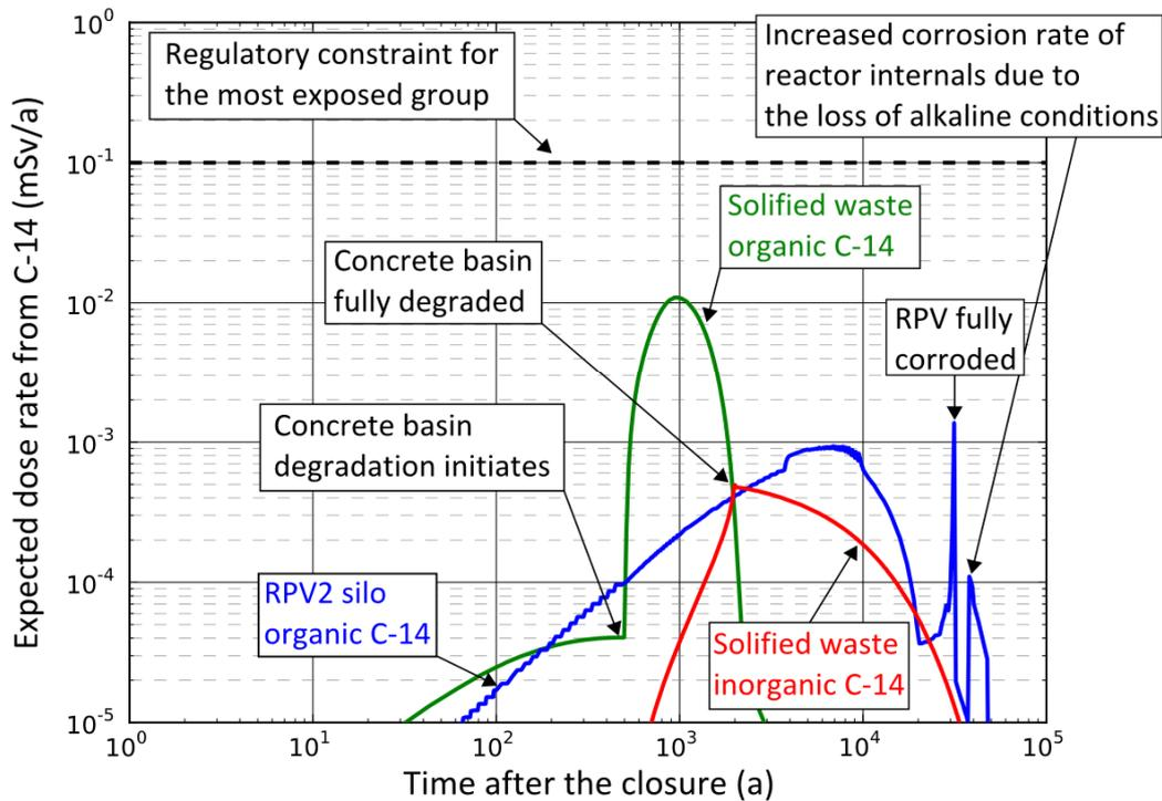
**Figure 2: The doses arising from solidified waste cavern and reactor pressure vessel silo 2 (RPV2), calculated using conservative parameter values. The dose rates from the both reactor pressure vessel silos are almost identical and hence only RPV2 results are shown. The well probability of 10 % has been taken into account in the expected dose rate.**
