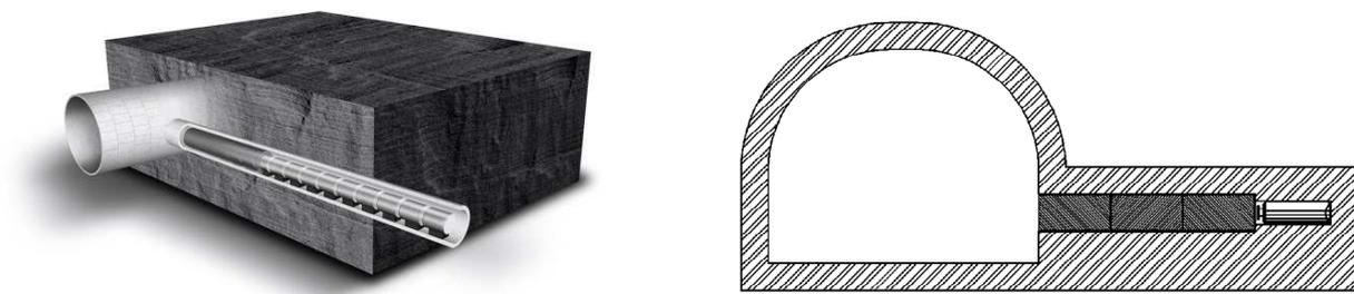
**Figure 3. Artist impression of the HLW waste in clay (left) and rock salt (right)**
