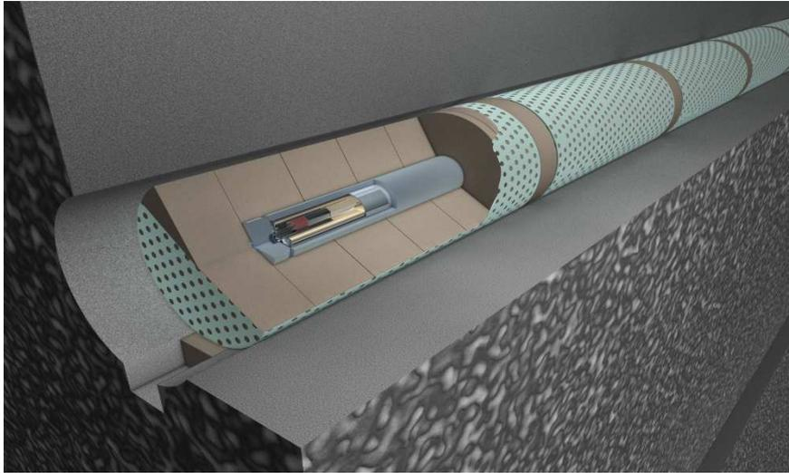
**Figure 1: Visualisation of the Czech DGR concept using horizontal boreholes**
