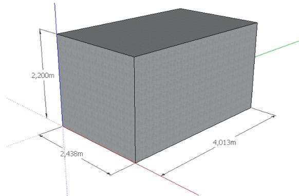
**Figure 1: Steel container considered for the analysis of C-14 migration from RBMK-1500 graphite waste**
