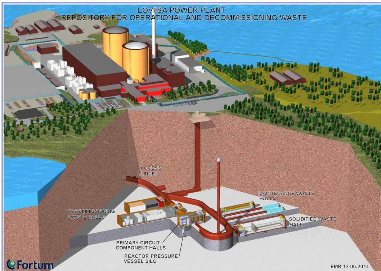
**Figure 1: The LILW repository located at Loviisa NPP site. The existing waste caverns of the operational waste are located on the right side of the connection tunnel, whereas the future decommissioning waste caverns are located on the left.**
