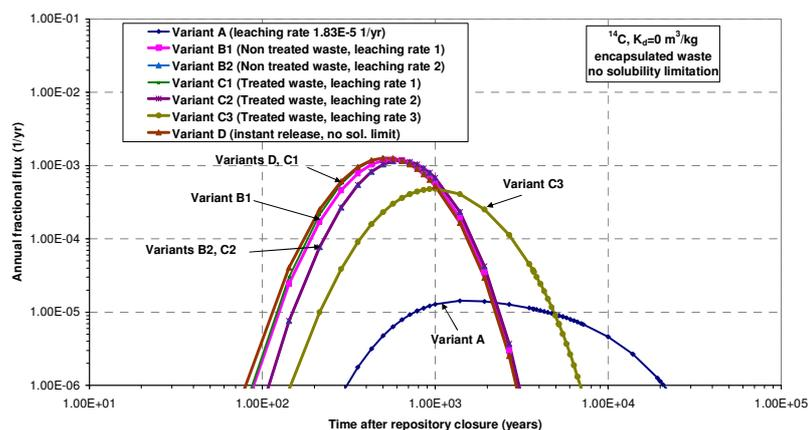
**Figure 5: Release of C-14 to the geosphere from one disposal container with not encapsulated waste (results of Case 1, sorption and solubility limit disregarded)**
