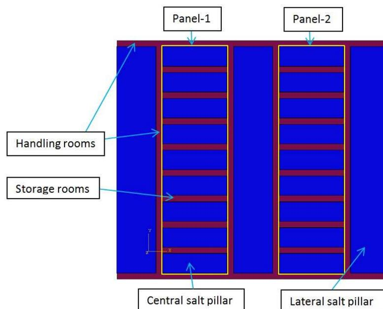
**Figure 2: Preliminary layout of geological repository (underground facility).**
