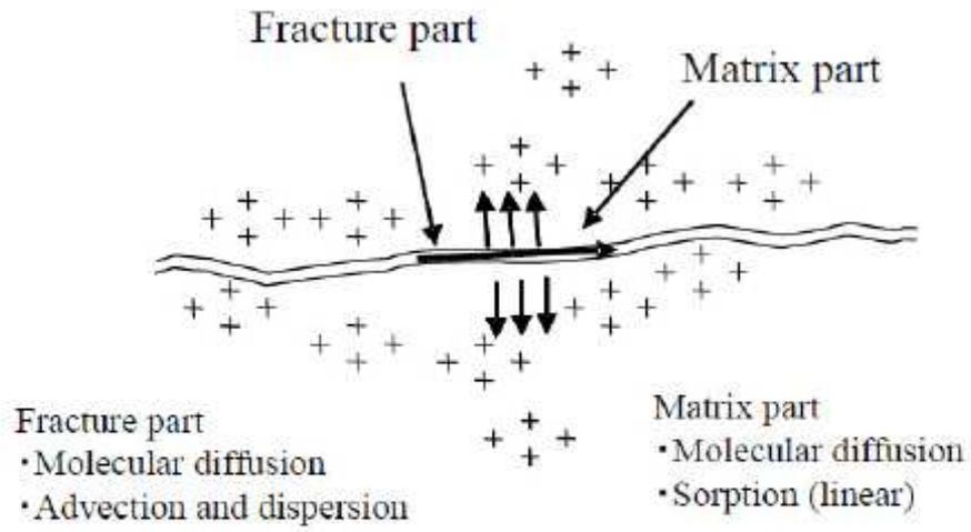
**Figure 7: Conceptual illustration of the radionuclide transport in the natural barrier (host rock).**
