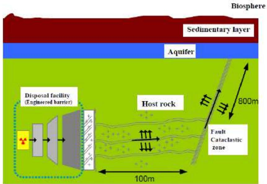
Figure 5: Overview of radionuclide transport pathway.
