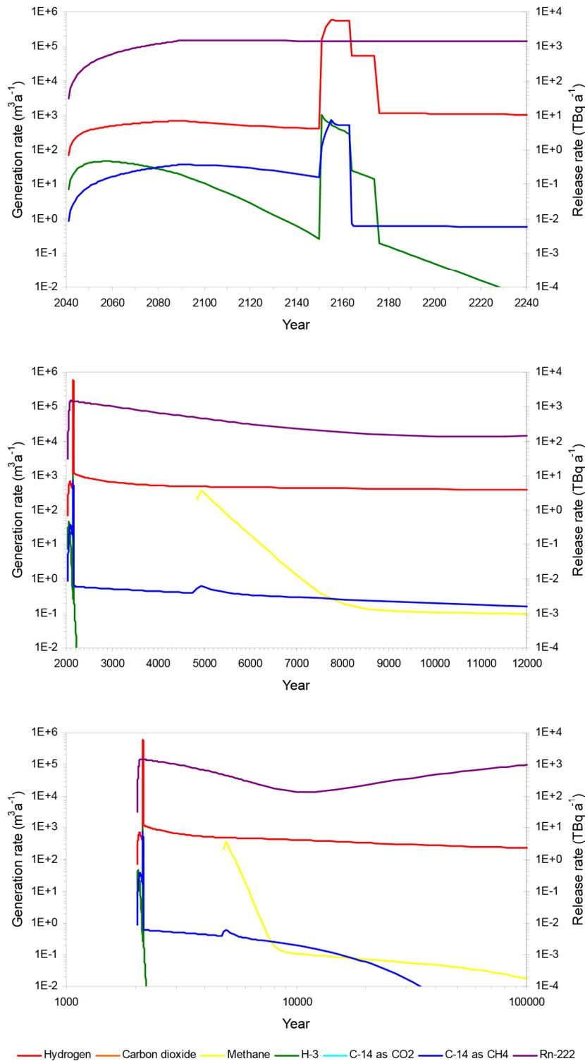
**Figure 3 Gas generation from the 2004 UILW inventory for the Reference case – plotted on various time scales. The bulk gases (i.e. H<sub>2</sub> and CH<sub>4</sub>) are plotted vs. the left-hand axis, and the active gases (i.e. <sup>3</sup>H, <sup>14</sup>CH<sub>4</sub> and <sup>222</sup>Rn) are plotted vs. the right-hand axis. CO<sub>2</sub> reacts with cement [9].**
