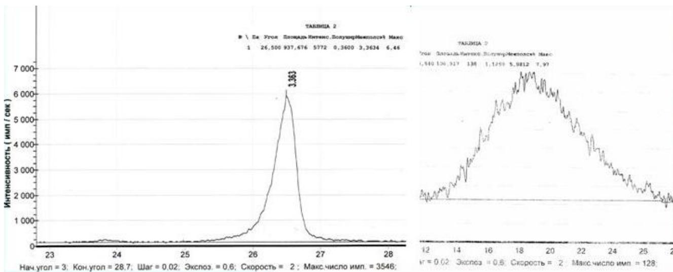
The 001 diffraction in GI, gradually disappeared with an increasing reaction time, implying the expansion of graphite layers.
