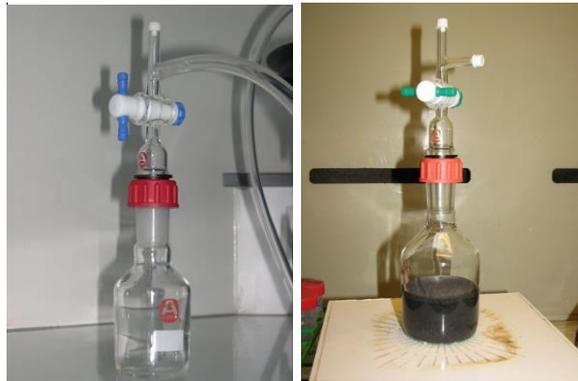
**Figure 2. Gastight glass containers (without and with graphite powder) for leaching experiments**
