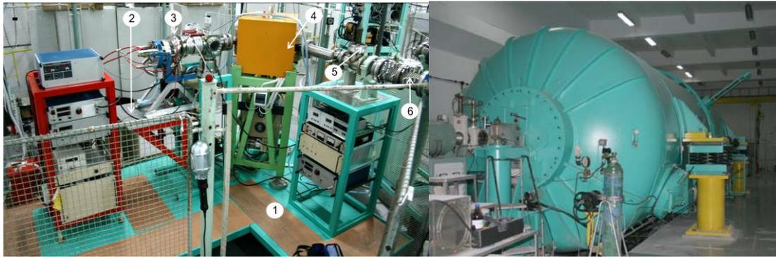
**Figure 8a:** Left: the Injector deck of the 9 MV tandem AMS facility in Bucharest: (1) Injector platform polarized at -100 kV, (2) second platform polarized at -30kV in respect to the first platform, (3) the ion source (40 NC-SNICS ), (4)  $90^\circ$  analyzing magnet, (5) slits and retractable Faraday cup, (6) pre-acceleration NEC tubes. Right: the tandem 9 MV FN accelerator.
