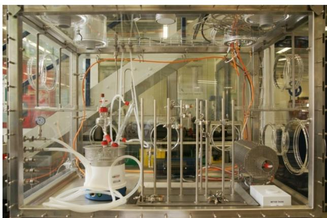
**Figure 11** Horizontal view with the heating element and furnace with the additional shielding for protection against hot areas during operation of the furnaces.
