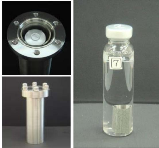
**Figure 16 External view of outer vessel (left) and cladding immersed in glass vessel (right) for long-term static leaching test.**
