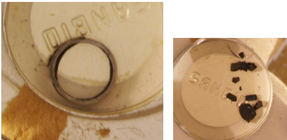
**Figure 8 (left): Dark film on inner surface seen after first acid clean. Little difference is seen after second acid clean; (right): pieces of fuel after defueling.**
