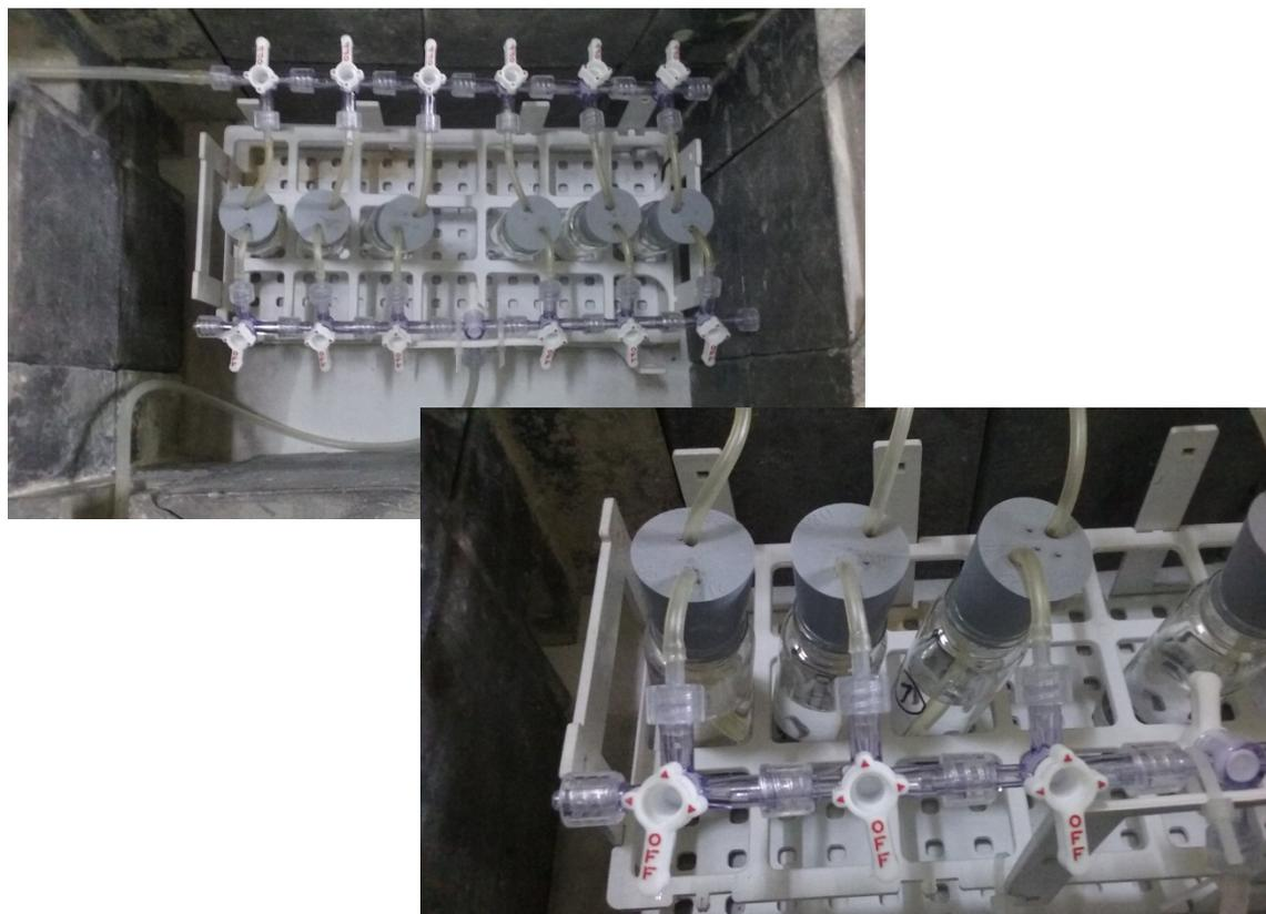
**Figure 14** View of the six glass bottles used in the leaching tests
