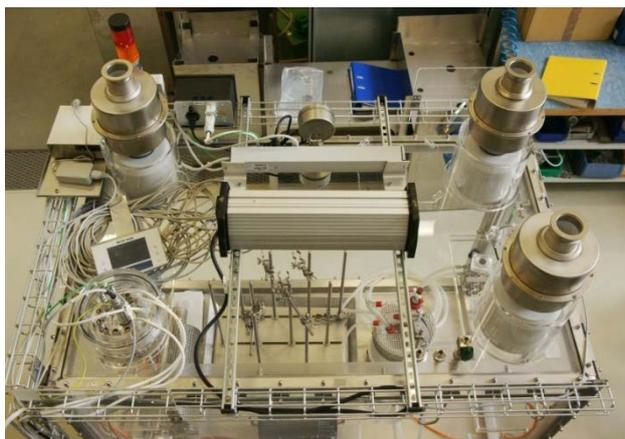
**Figure 10** Photograph showing the additional work on the glove box roof: glove box filter system and glove box lighting placed on top.
