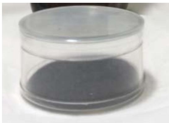
**Figure 2.3.3. Irradiated graphite sample subject to gamma spectrometry analysis**
