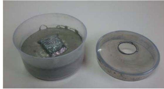
Figure 2.7.2. Cemented graphite sample.
