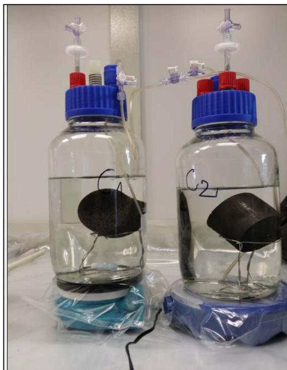
**Figure 2.3.4. Photograph of leaching set-up for anaerobic conditions**
