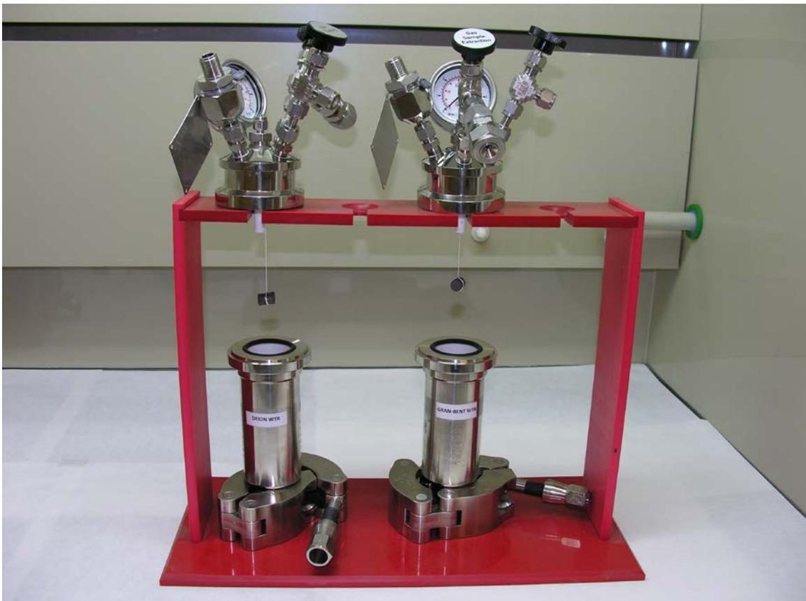
**Figure 2.7.5. Leaching containers for deionized water and granite-bentonite water.**
