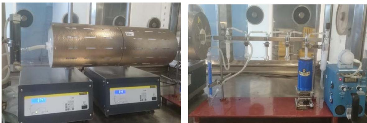
**Figure 2.8.5. Pictures of the experimental apparatus. (left) - tubular furnace tandem; (right) –  $^3\text{H}$  and  $^{14}\text{C}$  retention system**
