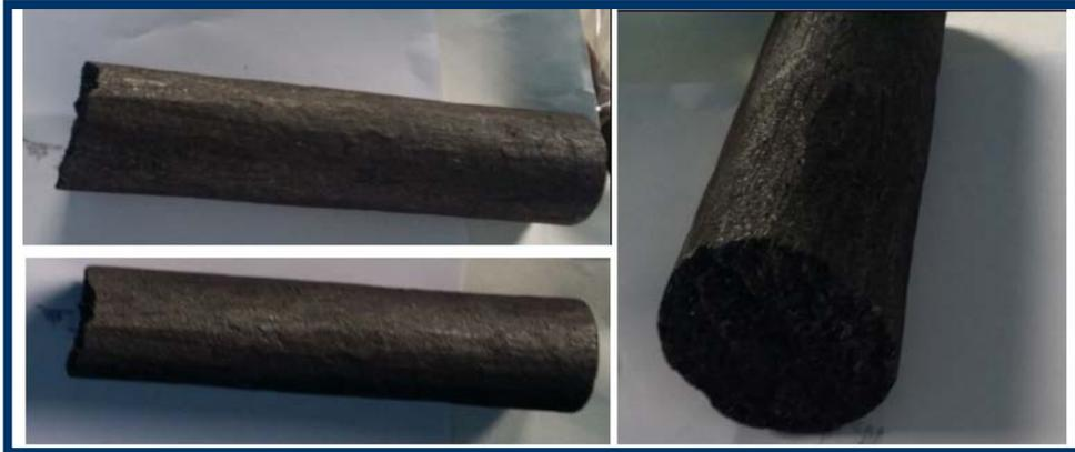
**Figure 2.3.1. Physical appearance of the i-graphite cylindrical bar from TRIGA thermal column**
