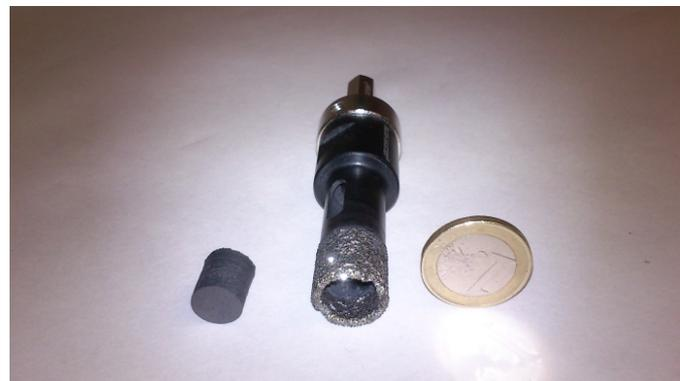
Figure 2.7.3 (Above). Graphite core 11 mm x 12 mm ( $\text{\O} \times \text{H}$ ) and diamond core drill 14 mm  $\text{\O}$ .
