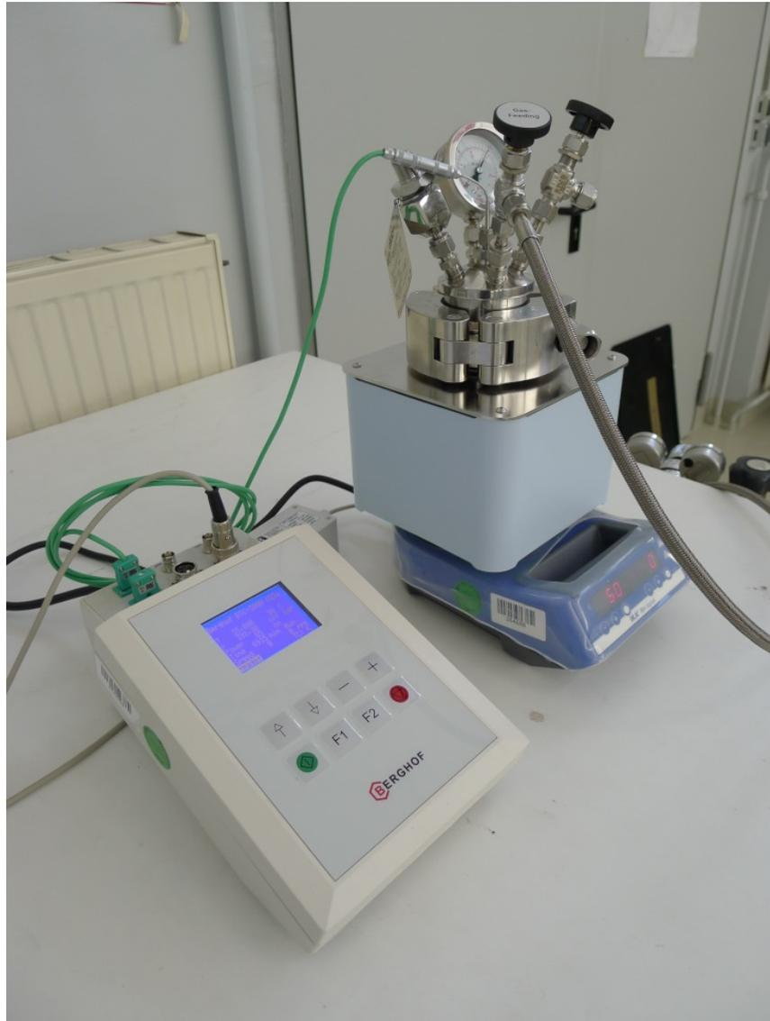
**Figure 2.6.4: An assembled reactor vessel (Berghof GmbH) for leaching test with nuclear graphite.**
