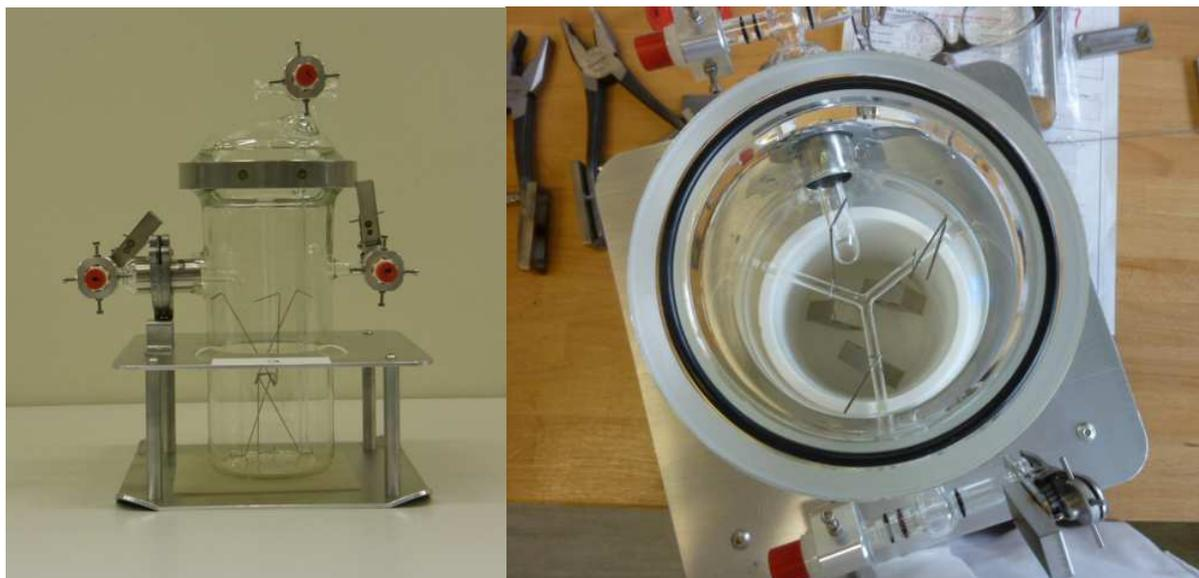
**Fig. 2 Leaching container (left) and a detail of the fixed CT specimens in the container (right)**
