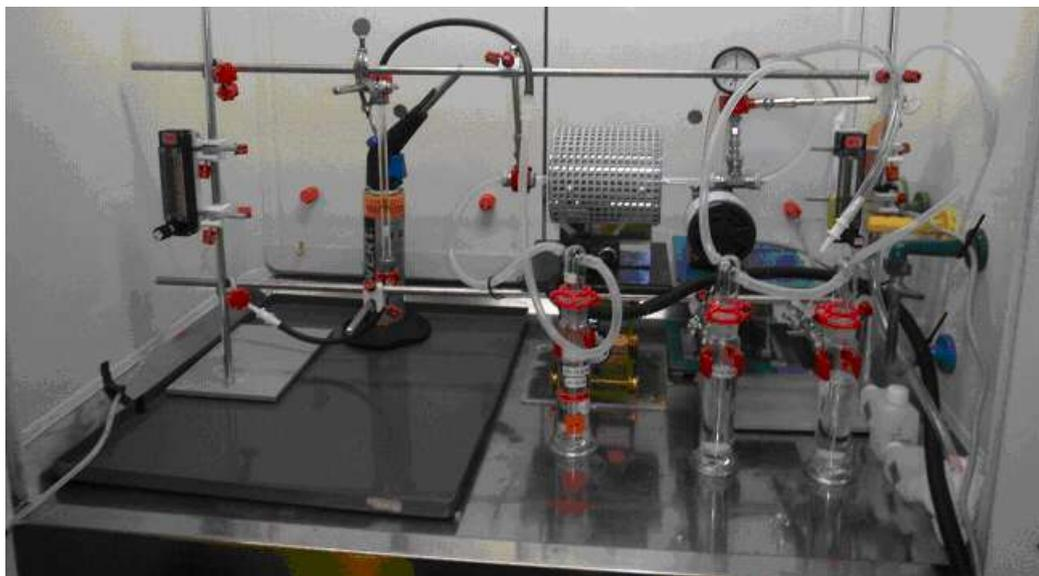
Figure A9-3. System set-up used for the combustion of spent ion exchange resins. The gas washing bottles are designated by 1–3 in the text.
