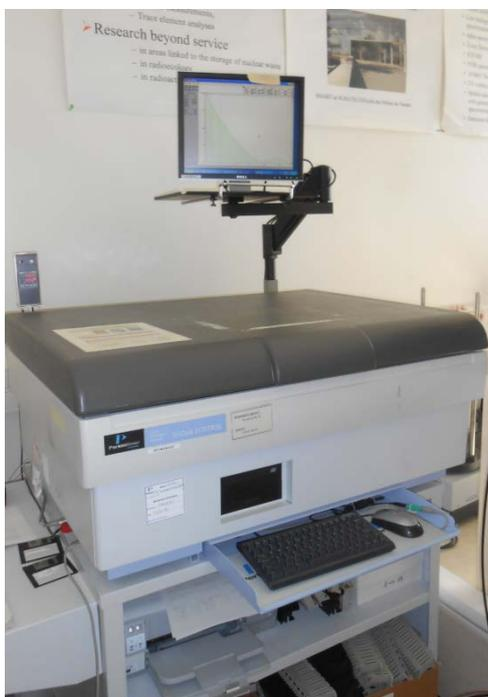
**Figure 8: Tri-Carb analyzer used for C-14 carboxylic acids analysis in the collected fractions**
