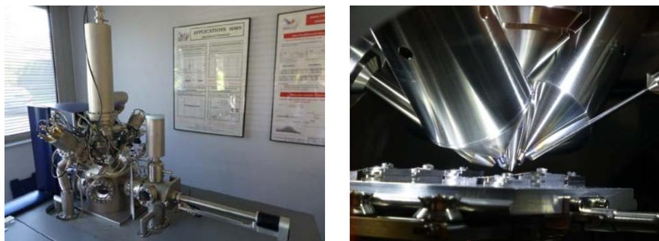
**Figure 5:** Pictures of the IONTOF ToF-SIMS V and the ionisation chamber
