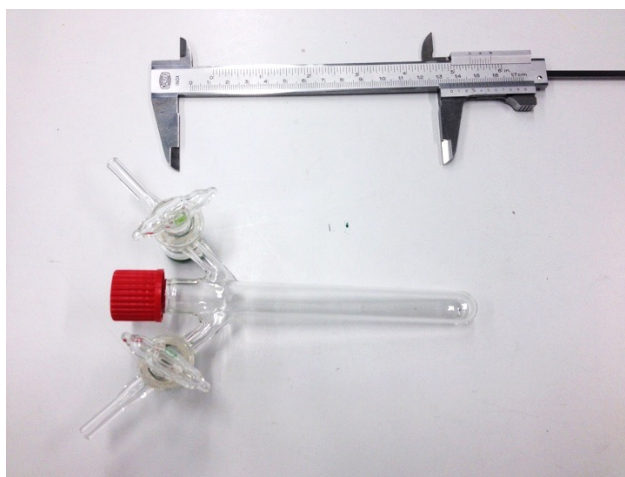
Figure 3. Example of vial used for the storage experiments of small FZJA/B samples
