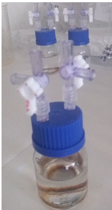
Figure 4. The glass vessels adapted for desorption tests.
