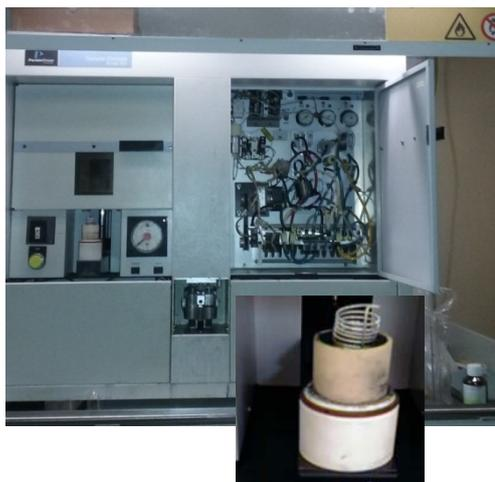
**Figure 1. The experimental device used for total  $^{14}\text{C}$  measurements in liquid samples**
