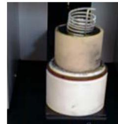
**Figure 2. Non-catalytic oxidation and collection of carbon for total  $^{14}\text{C}$  measurements in liquid samples**
