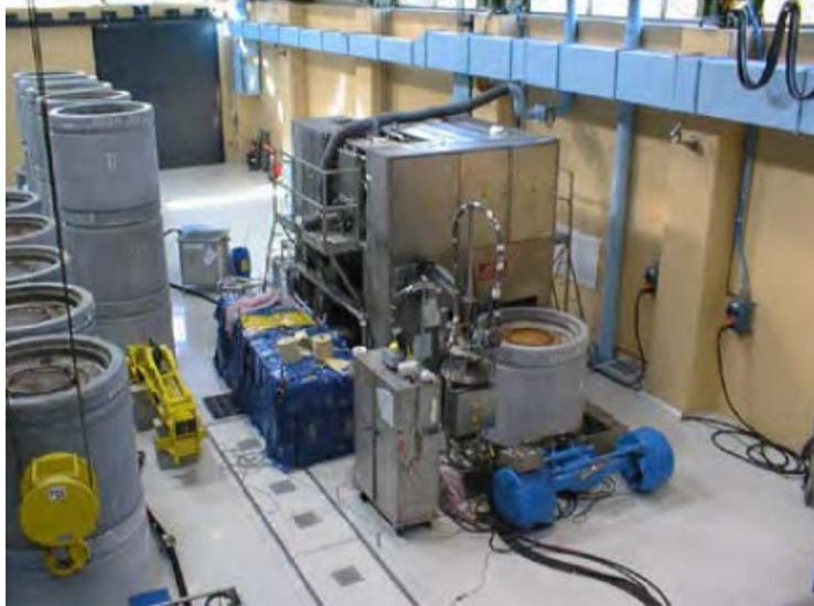
**Figure 9. Mobile unit used for SIERs conditioning on-site.**
