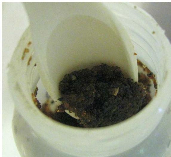
**Figure 2. SIER from Dukovany Nuclear Power Plant operation**
