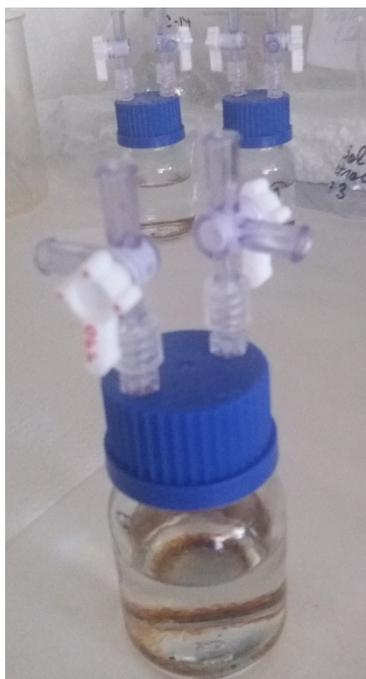
**Figure 6. The glass vessels used in desorption tests [BUCUR *et al.*, 2017].**
