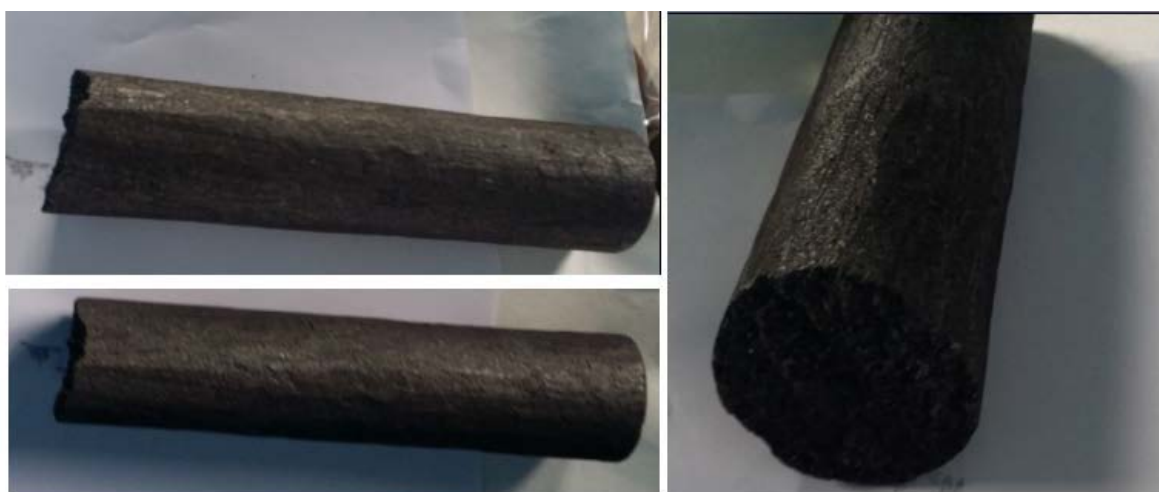
Figure 1. The irradiated graphite cylindrical bars used to cut intact samples for leaching experiments and powder samples to measure the radionuclide content
