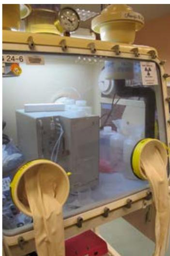
**Figure 13: TOC analyzer in a glove box**
