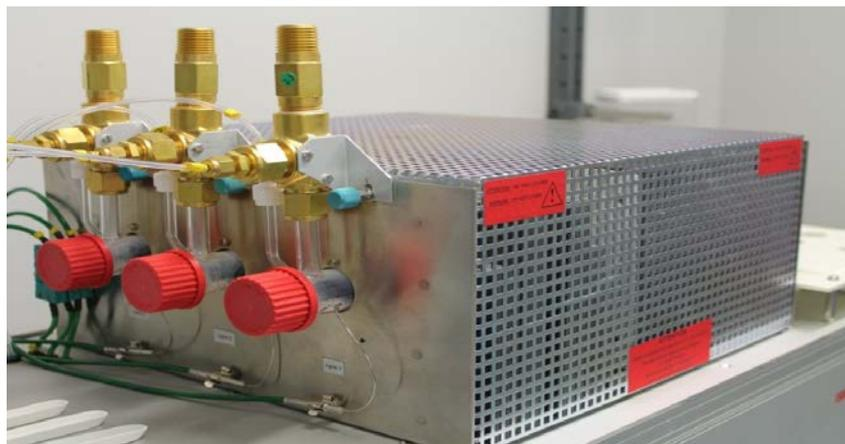
**Figure 8: Tri-tube pyrolysis furnace.**
