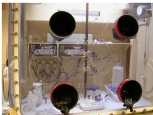
**Figure 15 : Ionic chromatography in glove box**
