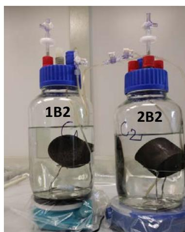
**Figure 2.3.4. Photo of the leaching set-up for anaerobic conditions**
