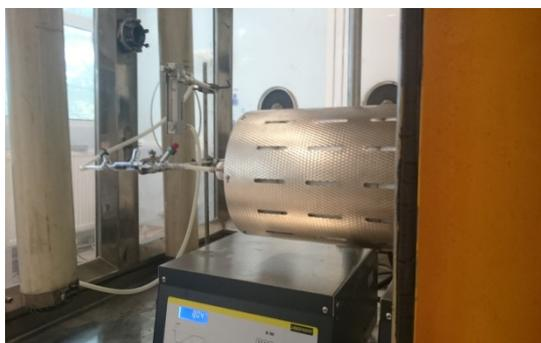
**Figure 2.8.13:** Apparatus for C-14 and H-3 retention
