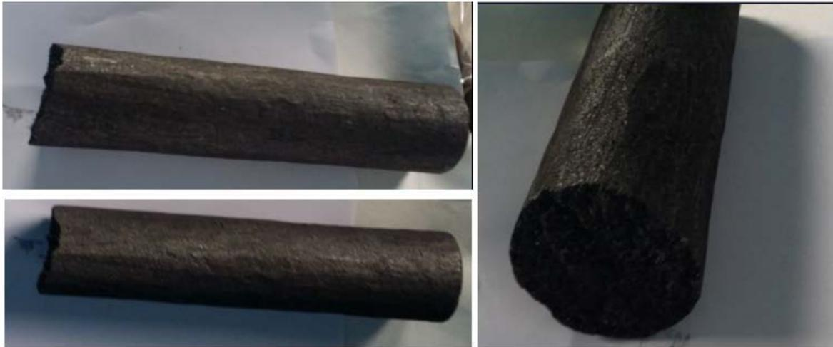
**Figure 2.3.1. The irradiated graphite cylindrical bars used to cut intact samples for leaching experiments and powder samples to measure the radionuclide content**
