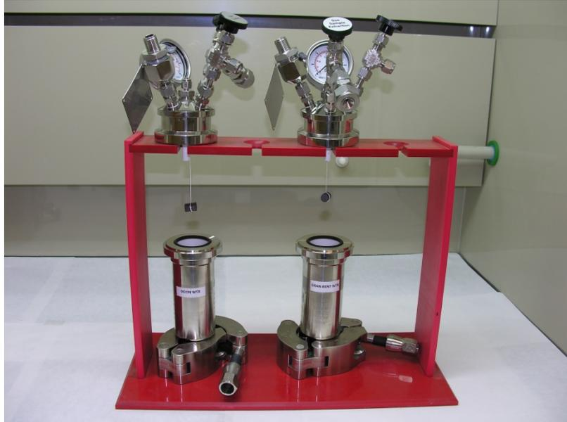
**Figure 2.7.1. Leaching containers for deionized water and GBW.**
