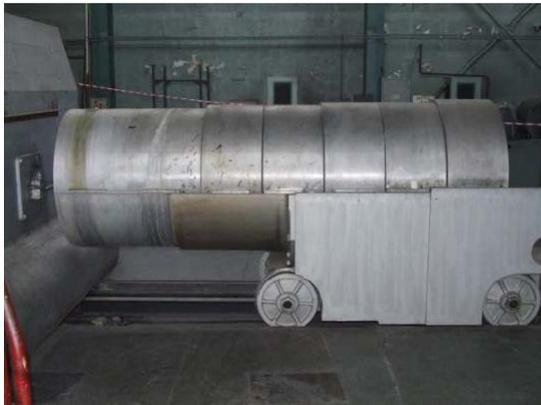
**Figure 2.8.2** Thermal column
