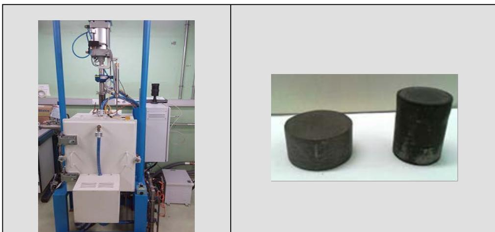
**Figure 2.7.4. Hot Press (ALD-France (FNAG) Technology) and IGM specimens**
