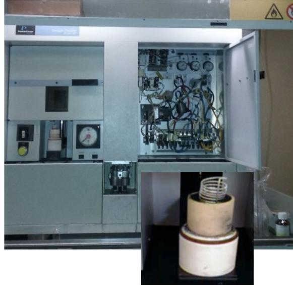
**Figure 2.3.5. The experimental device used for total  $^{14}\text{C}$  measurements in liquid samples**
