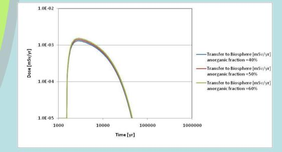
Variations of the congruent release of C-14 from Zy claddings do not show impact on the maximum dose, which is practically given by the IRF. The impact of different corrosion rates considered for the sensitivity analysis can be
