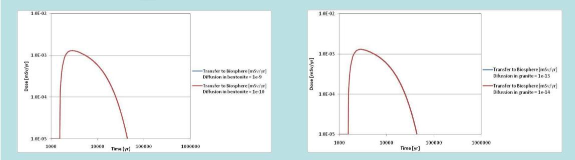
No significant influence has been found for the increase with one order of magnitude of the diffusion coefficients in bentonite and granite compared to the reference case, as long as the fractures remain the most effective transport pathway for radionuclides.
