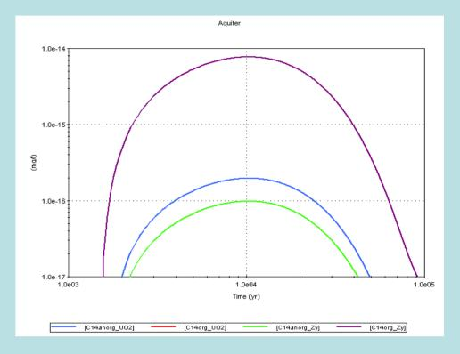
Due to the advective flow through the fractures, the maximum C-14 concentration in the aquifer is reached at 1100 years after canisters failure (left), while the diffusive component through granite which represents the larger part of the C-14 inventory, reaches the maximum release at 9800 years (right)
