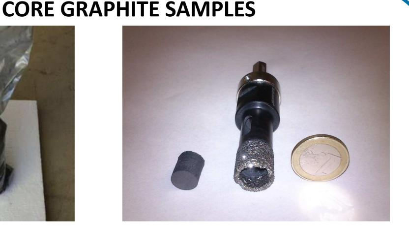
To the right core - drilled sample of ca. 2 g and 11 mm x 12 mm (Ø x H) from Vandellós I sleeve graphite (UNGG reactor). Bulk sample to the left.
