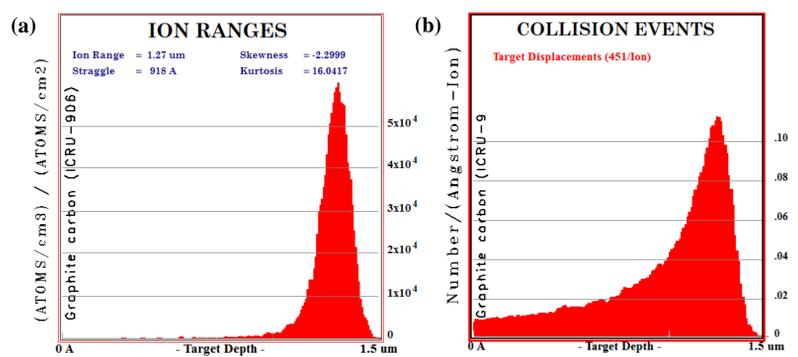
**Fig. 4.** 700 keV  $^{12}\text{C}^+$  ion implantation parameters according to SRIM: (a) the projected range of implanted ions; (b) the damage profile.
