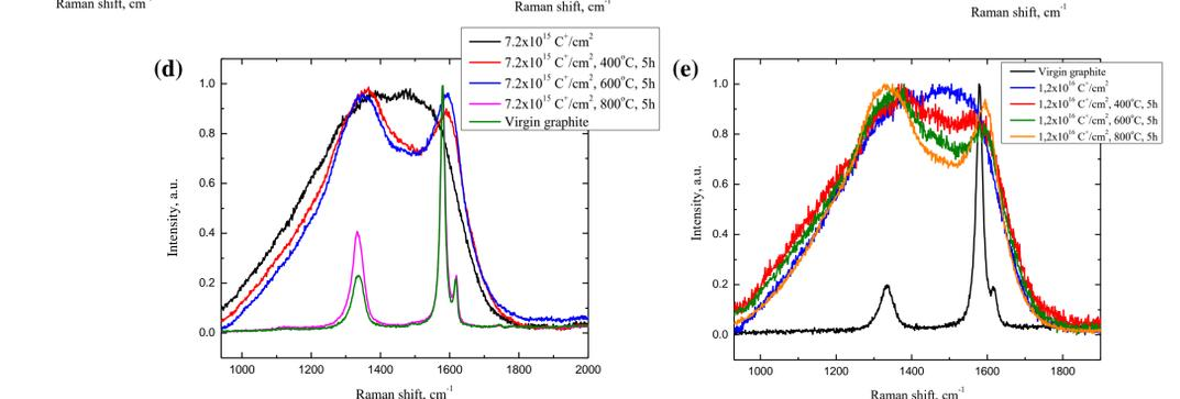
**Fig. 5.** Raman spectra of raw RBMK-1500 stack graphite samples (a) implanted at a fluence of (b)  $1.2 \times 10^{15}$  ions/cm<sup>2</sup> (c)  $3.5 \times 10^{15}$  ions/cm<sup>2</sup> (d)  $7.2 \times 10^{15}$  ions/cm<sup>2</sup> (e)  $1.2 \times 10^{16}$  ions/cm<sup>2</sup> and subsequently annealed at various temperatures ranging from 400°C to 800°C for 5h.
