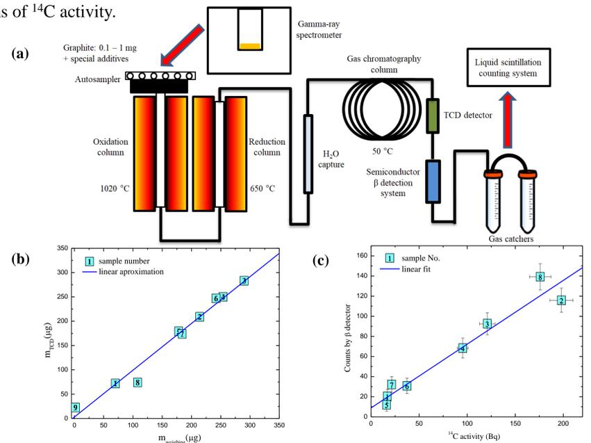
**Fig. 2.** (a) Rapid system for  $^{14}\text{C}$  specific activity determination in the sample. (b) The correlation of the graphite sample mass as determined by two independent methods: weighing and combustion in the elemental analyzer. (c) Correlation between LSC and semiconductor detector data.
