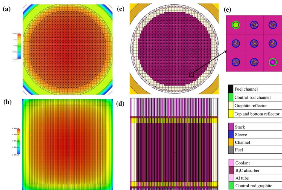
**Fig. 1.** (a) Neutron flux distribution in the RBMK reactor graphite horizontal and (b) vertical cross sections. (c) Horizontal cross section full scale reactor core; (d) vertical cross section of reactor core with bottom, top reflectors, metal plates and cooling tubes system on the top. (e) Magnified view of RBMK-1500 core fragment (3x3) with fuel assemblies, inserted and extracted control rods.
