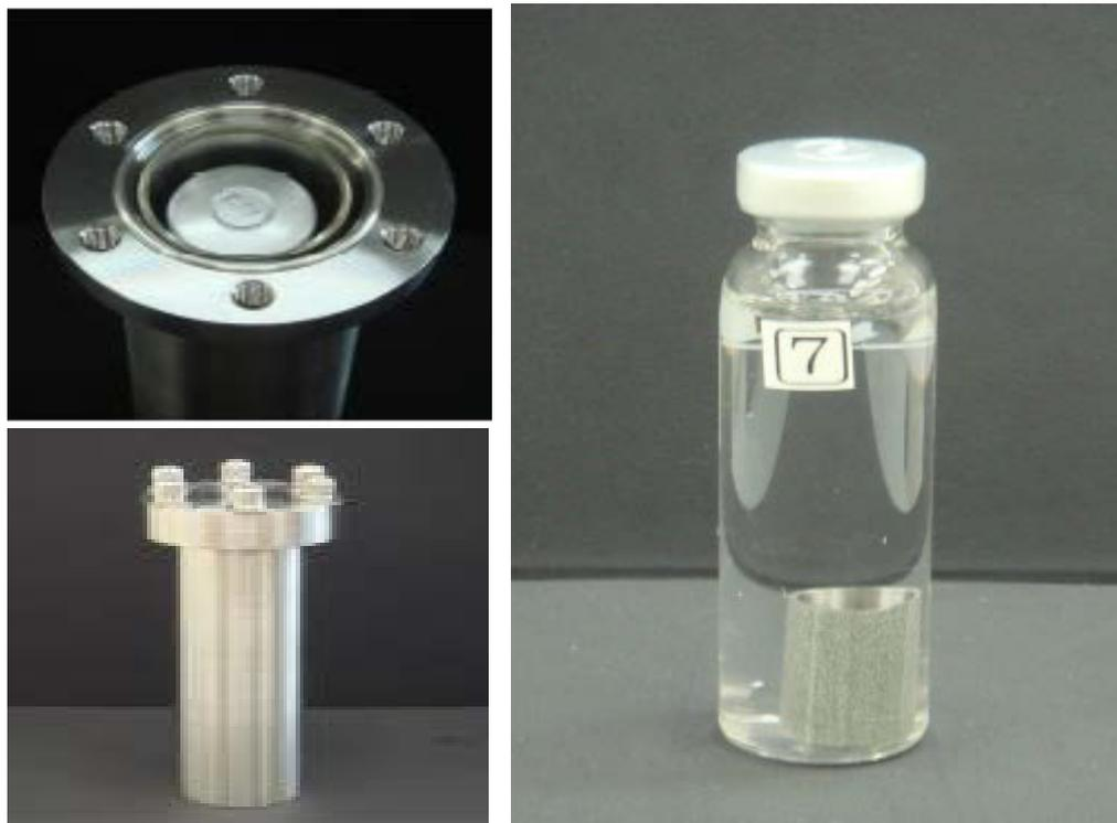
**Figure 25** External view of the outer vessel (left) and cladding with external oxide immersed in the glass vessel (right) for long-term static leaching tests.
