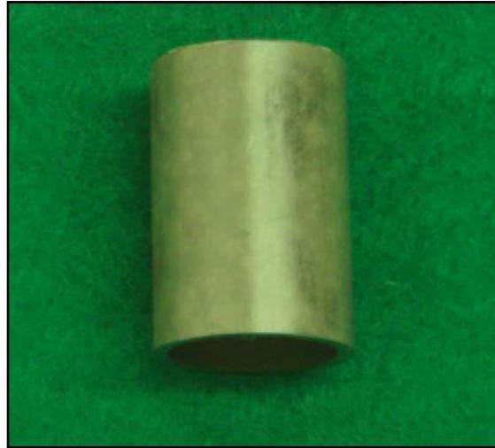
Figure 15 Irradiated Zircaloy-2 (BWR STEP III) after HNO<sub>3</sub>washing.
