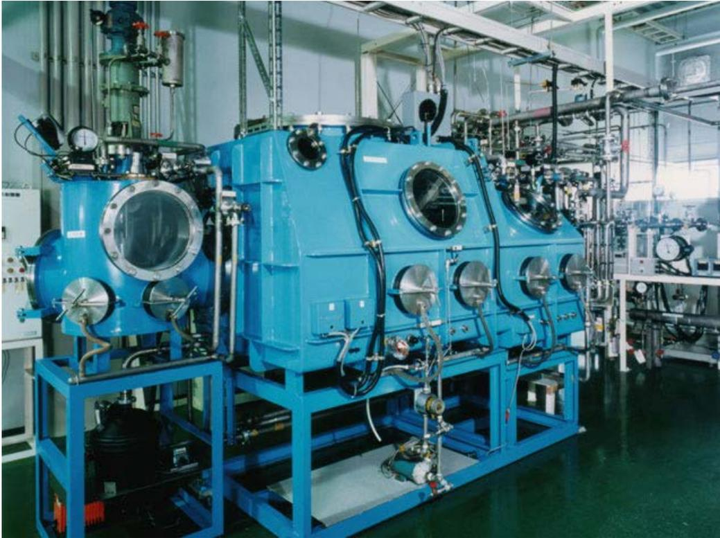
Figure 5 Glove box for preparation of glass ampoule.
