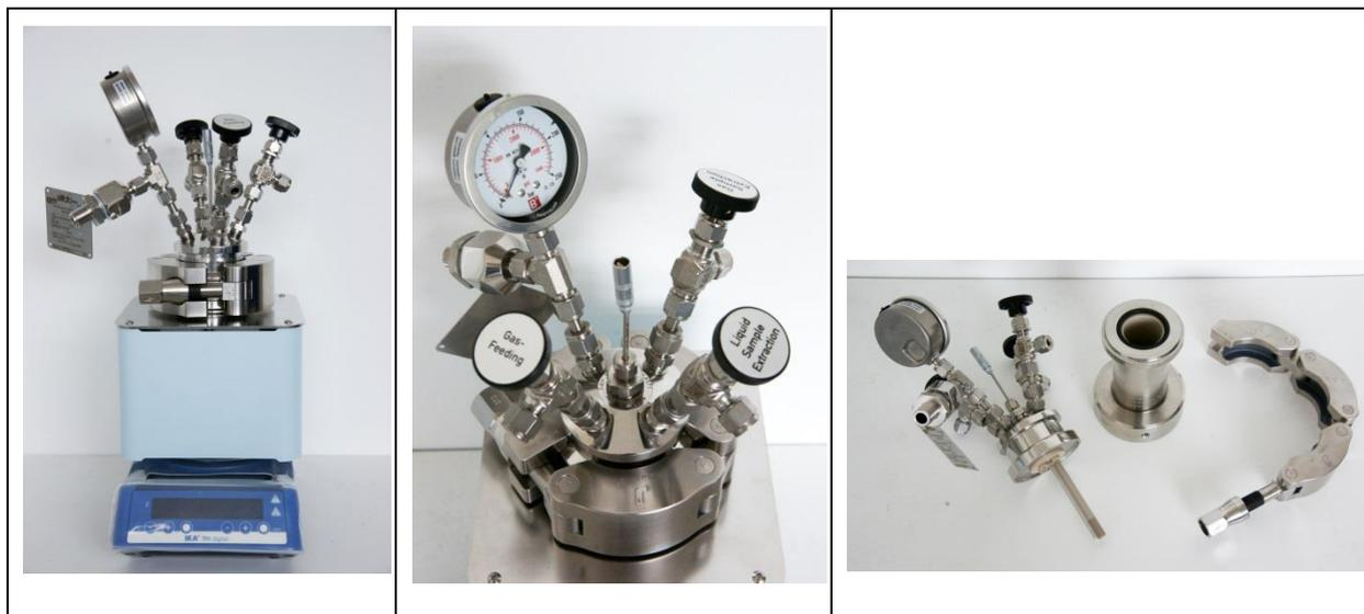
**Figure 3.6: Second Autoclave with heating mantel**
