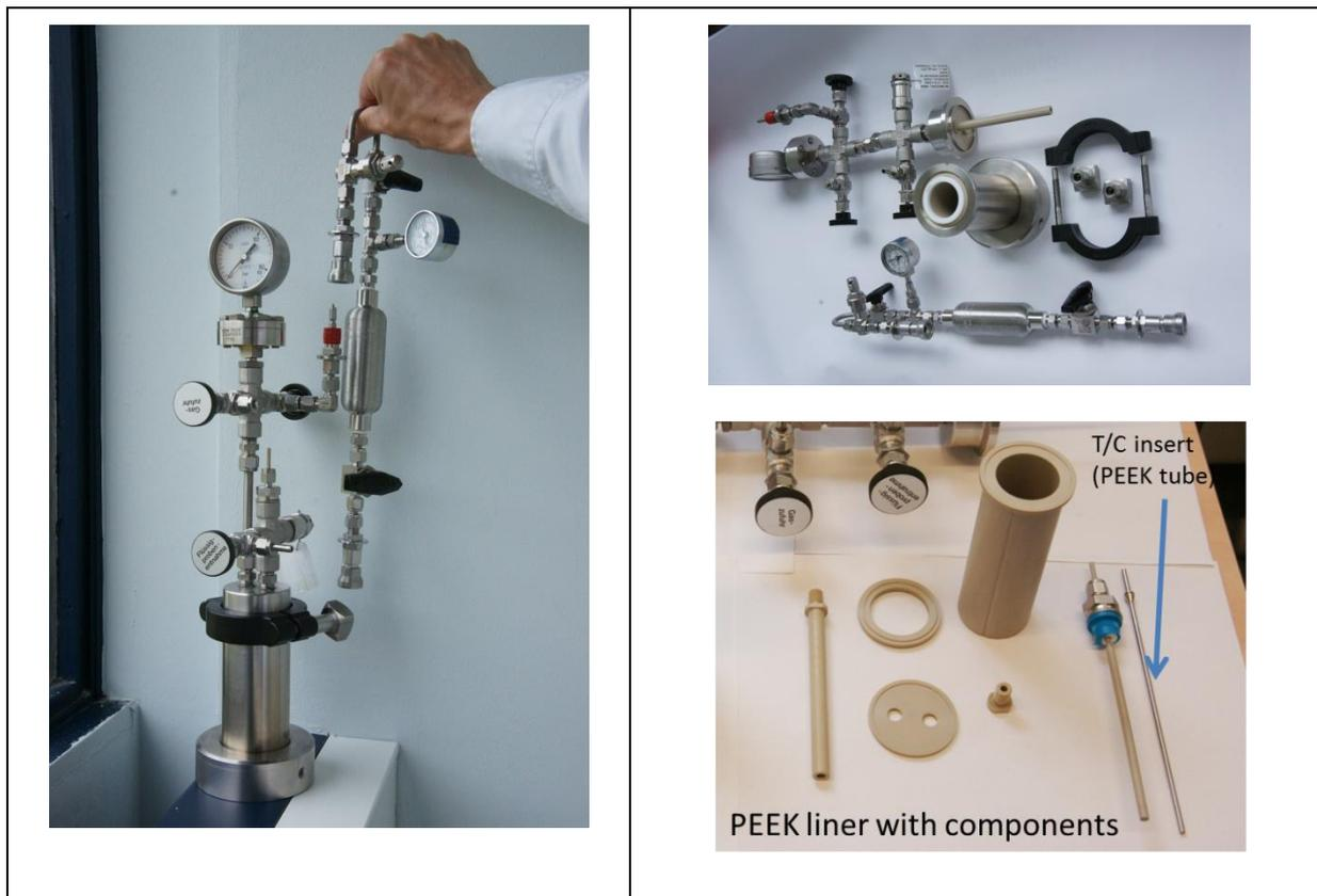
**Figure 3.5: Berghof autoclave (left) with its gas sampling vessel, and a view of its internal components (right)**
