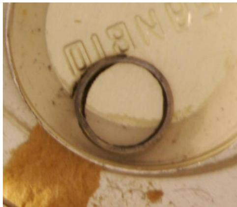
**Figure 2.1 Visual inspection of the Zry cladding sample**
