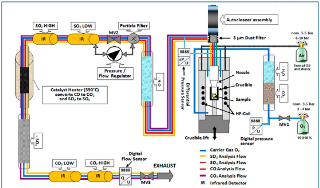
Figure 3.2 ICARUS device operating principle
