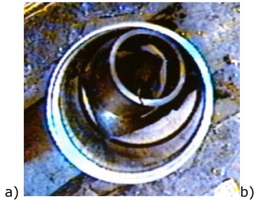
**Figure 2.2: NIMPHE carbide fuel cladding following defueling. A dark thin oxide layer is observed before cleaning.**
