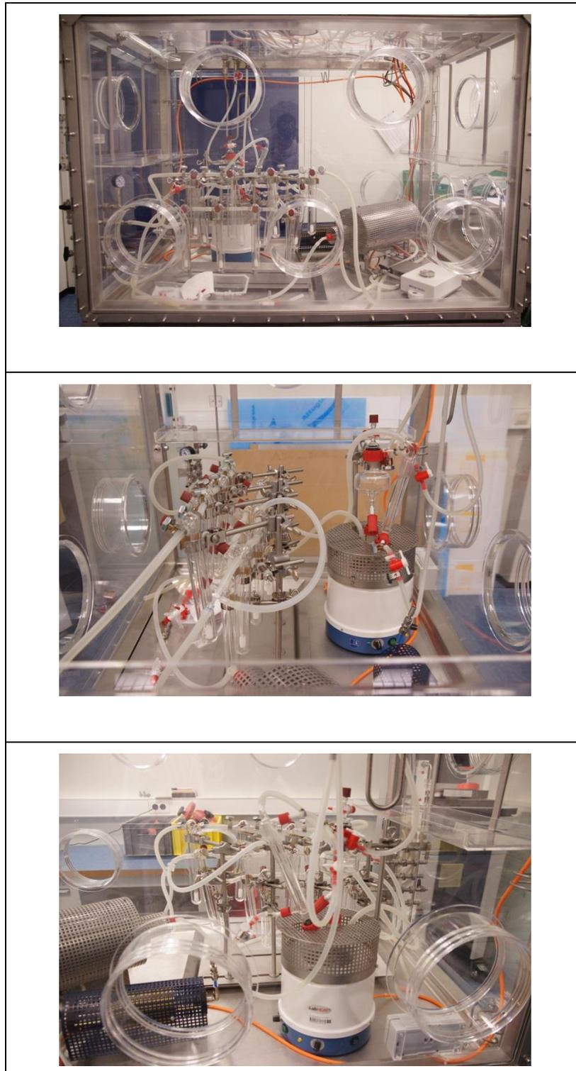
**Figure 3.8: Completed Glove box for  $^{14}\text{C}$  sample preparation.**
