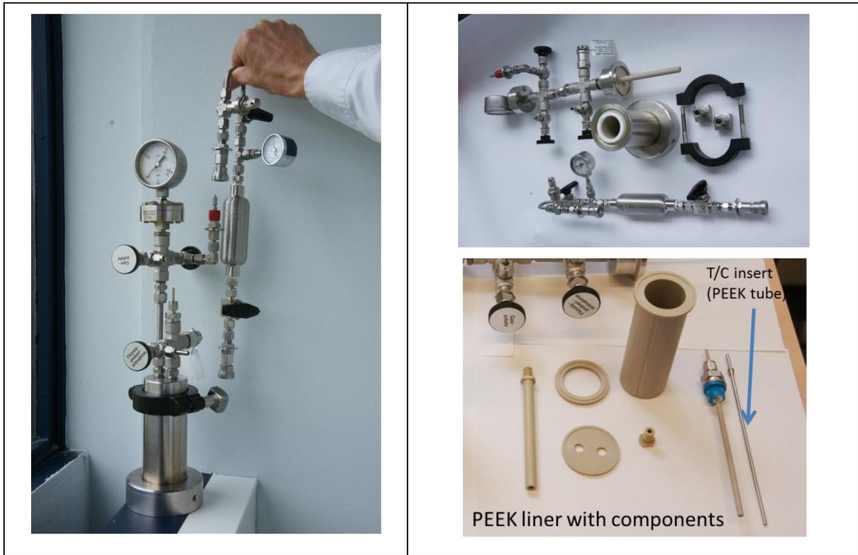
**Figure 3.5: Berghof autoclave (left) with its gas sampling vessel, and a view of its internal components (right)**
