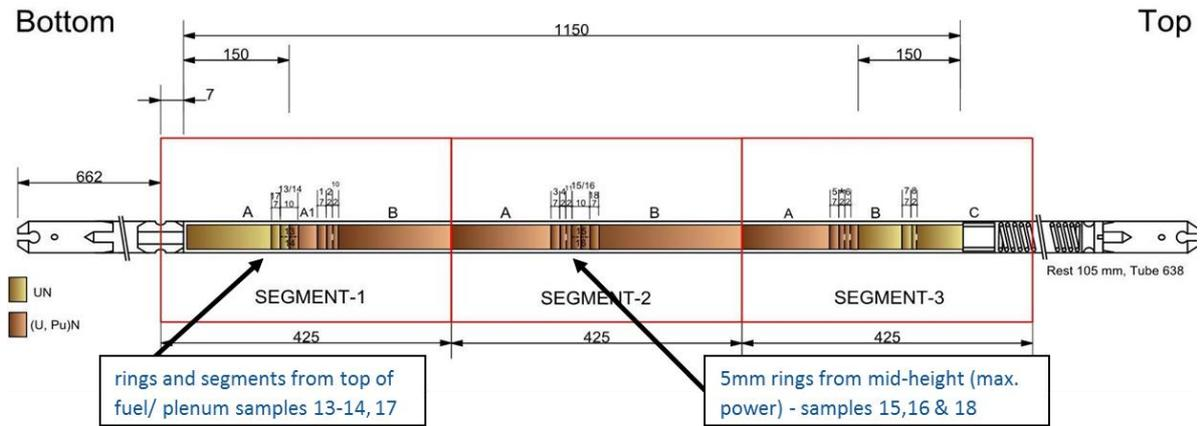
**Figure 2.1 Cutting plans for steel sample rings from NIMPHE 2 pins**
