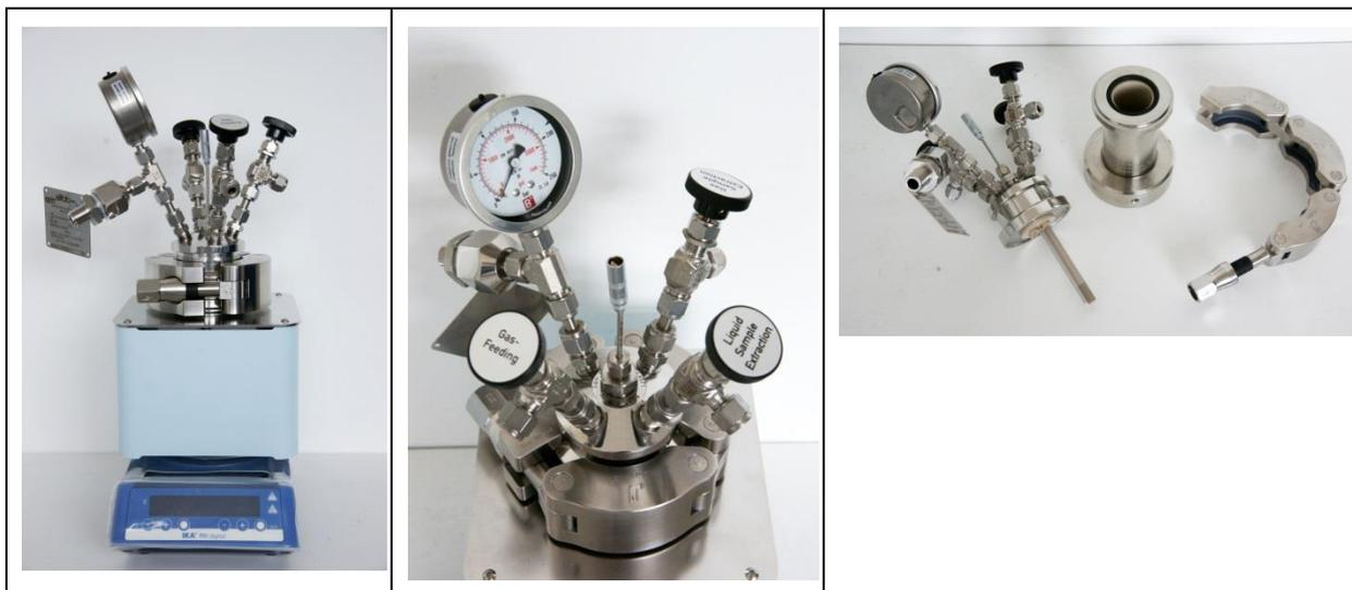
**Figure 3.6: Second Autoclave**
