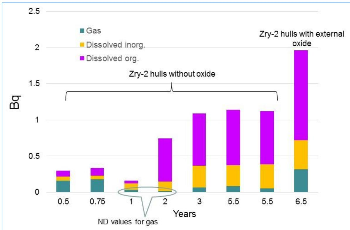
**Figure 7 C-14 measured on irradiated Zircaloy-2 (metal + oxide) and Zircaloy-2 (metal only)**
