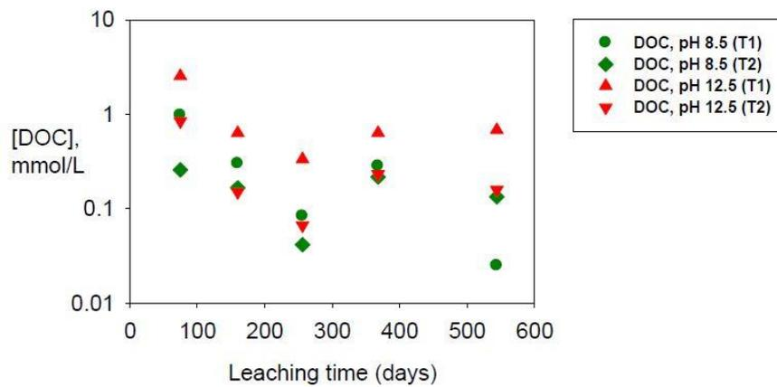
**Figure 5: Dissolved organic carbon (DOC) in the preliminary leaching tests of Loviisa steel in simulated groundwater at pH 8.5 and 12.5 as a function of leaching time. T1 represents tests with m/V= 50 g/100 mL and T2 tests with m/V= 25 g/100 mL.**
