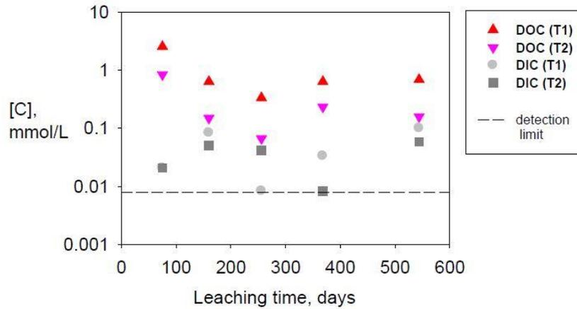
**Figure 4: Dissolved inorganic (DIC) and organic (DOC) carbon in the preliminary leaching tests of Loviisa steel in simulated groundwater at pH 12.5 as a function of leaching time. T1 represents tests with m/V= 50 g/100 mL and T2 tests with m/V= 25 g/100 mL.**
