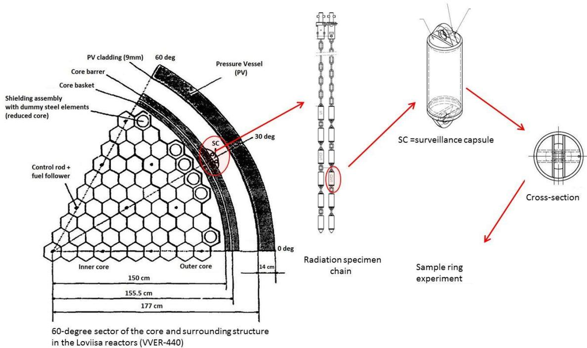
**Figure 2: Schematic drawing of the surveillance capsule and its position in the reactor (Pictures by Fortum Power and Heat Oy).**
