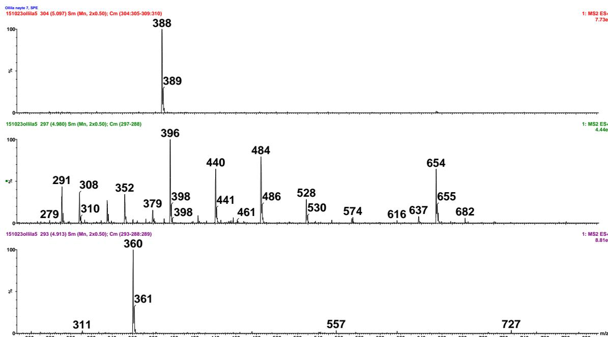
**Figure 10: The ESI-MS-spectra taken from the three peaks detected in the sample from Fe<sub>3</sub>C test (pH 12.5). Upper spectrum is a peak at the retention time of 4.91 min, middle at 7.98 min and bottom at 5.1 min.**
