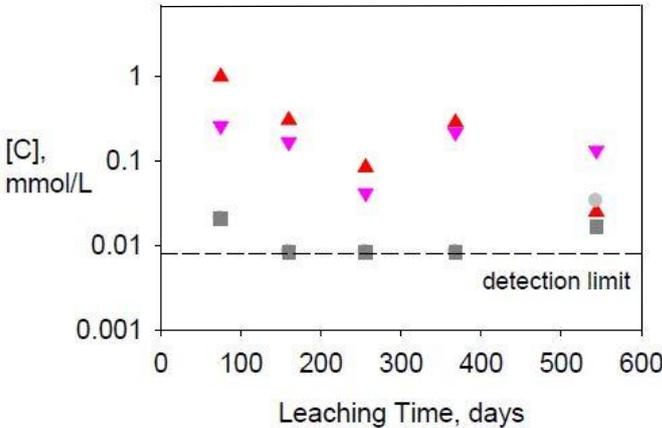
**Figure 6: Dissolved organic (red and pink) and dissolved inorganic (grey) carbon in the preliminary leaching tests of Loviisa steel in groundwater at pH 8.5 as a function of leaching time.**
