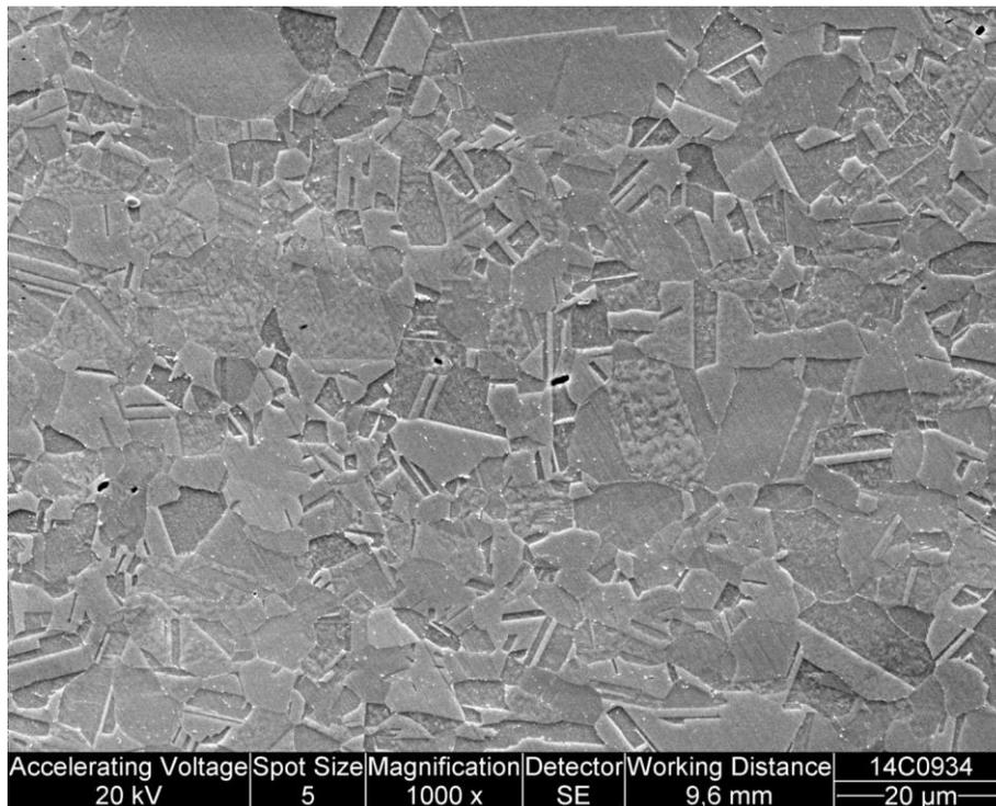
**Figure A1-1: SEM picture of the surface of Loviisa steel.**
