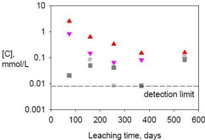
**Figure 7: Dissolved organic (red and pink) and dissolved inorganic (grey) carbon in the preliminary leaching tests of High carbon steel in groundwater at pH 8.5 as a function of leaching time**
