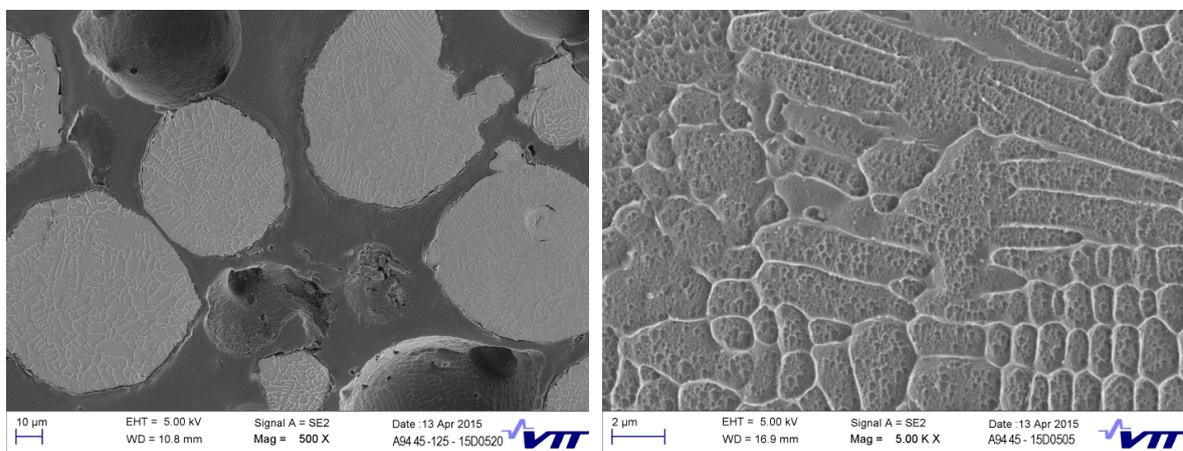
**Figure 1: SEM pictures of AISI316Ti steel powder after gas atomisation.**
