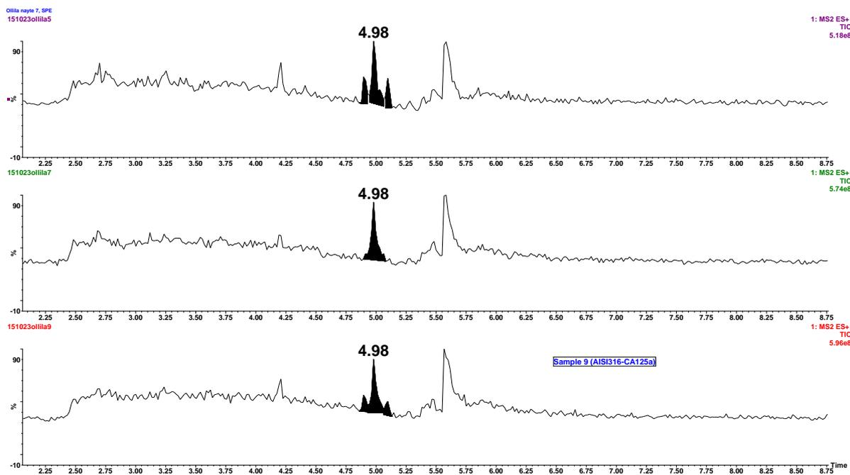
**Figure 9: The LC-MS total ion chromatograms (positive ionisation mode) of the samples after SPE.**
