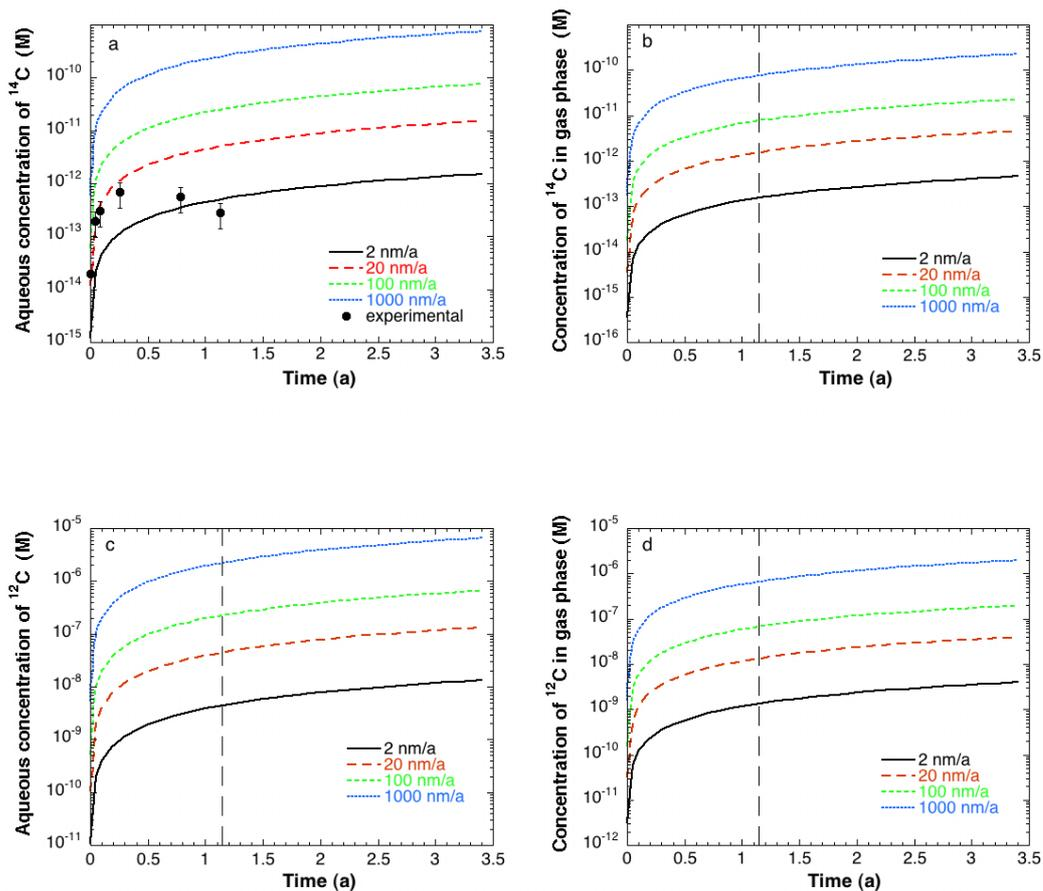
**Figure 8: Estimates of the total  $^{14}\text{C}$  (a/b) and stable carbon (c/d) concentrations in liquid and gas phase for the experimental set-up (see text) as a function of corrosion rate. The vertical broken line indicates 412 days reaction.**
