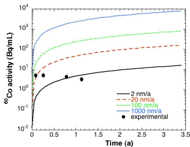
**Figure 7: Estimate of the  $^{60}\text{Co}$  activity in solution for the experimental set-up (see text) as a function of corrosion rate.**
