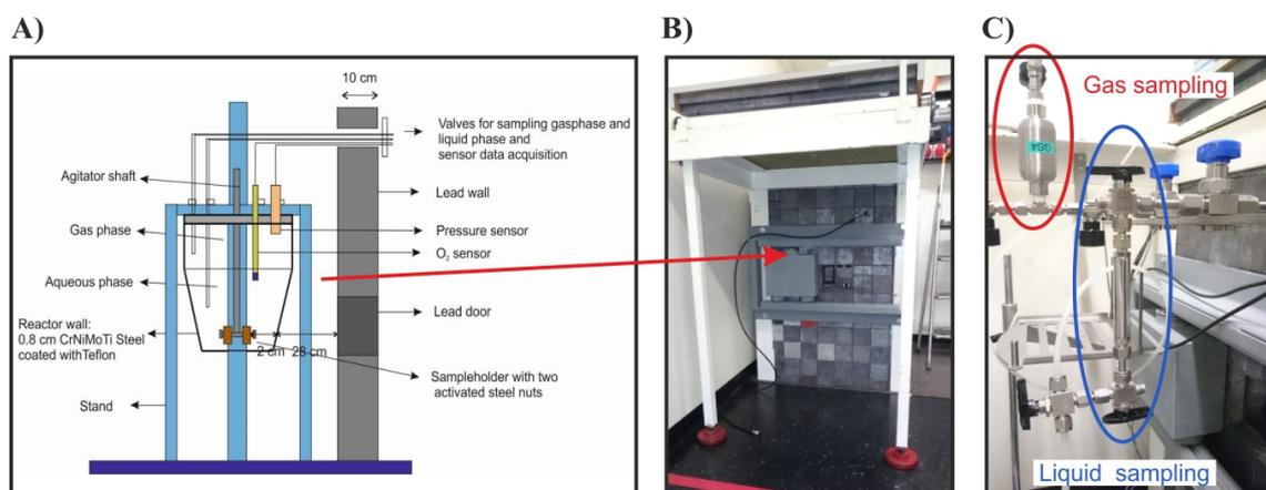
**Figure 4: A) Sketch of the reactor, B) picture of the lead shielding with door, and C) the sampling system for liquid and gaseous samples placed outside the shielding.**
