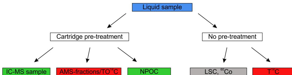
**Figure 6: Flow chart of sample treatment and analysis (see text).**
