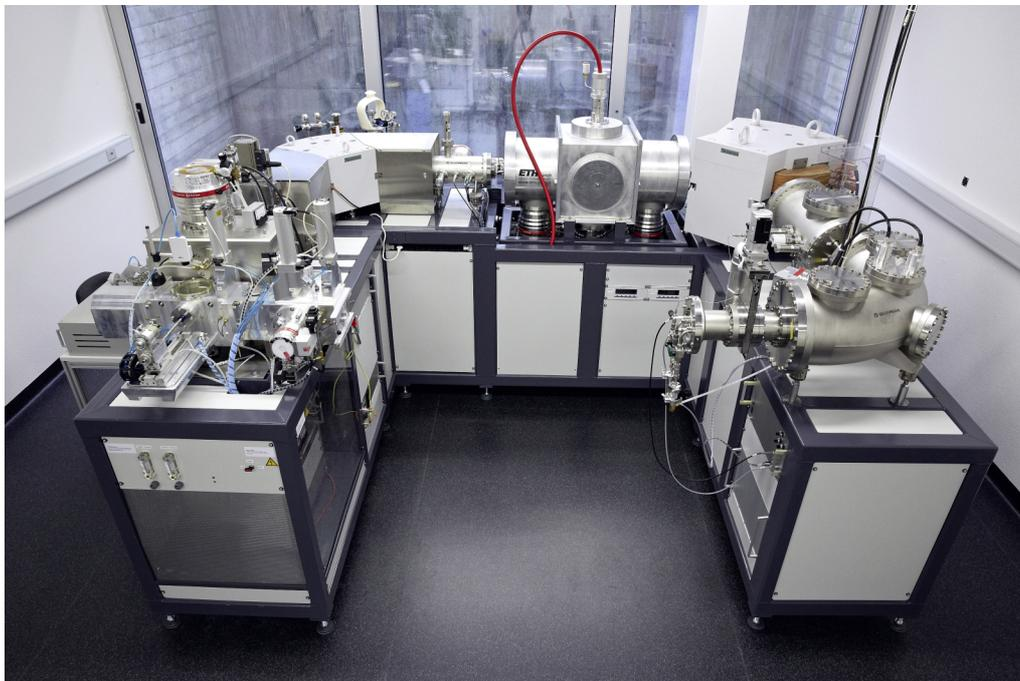
**Figure 2: Mini Carbon Dating System (MICADAS) at the Laboratory for the Analysis of Radiocarbon with AMS at the University of Bern (Switzerland).**
