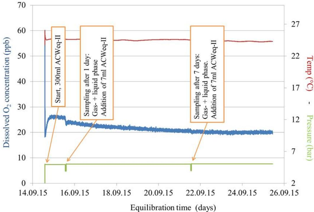
**Figure 5: Monitoring pressure (in green), temperature (in red) and O<sub>2</sub> concentration (in blue) during a first sampling test experiment.**
