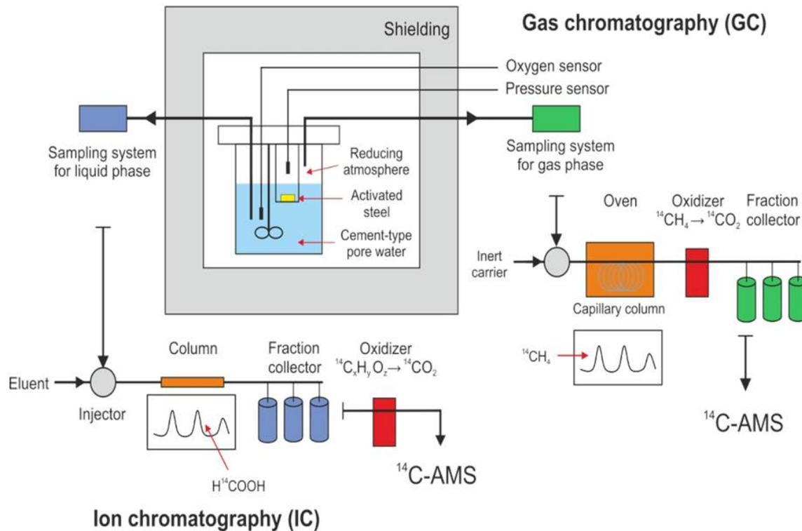
**Figure 1: Schematic representation of the set-up and analytical strategy for the planned corrosion experiment with irradiated steel at PSI.**
