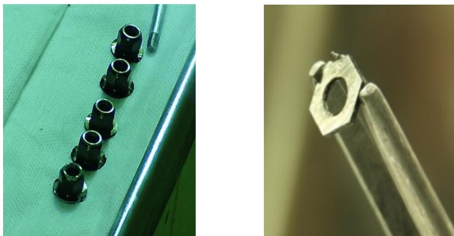
**Figure 3: Left: Irradiated steel nuts obtained from NPP Gösgen; Right: Specimens prepared from a steel nut for use in the experiments.**
