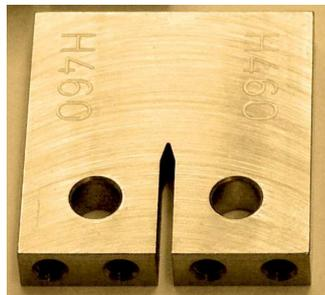
Figure 2 Photograph of a CT specimen
